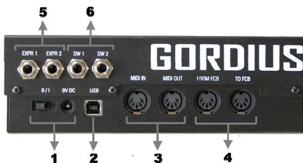
1. +9V DC power input with power switch
