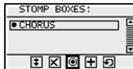
*With the "radiobutton" icon you can toggle the initial status of a stomp box*
