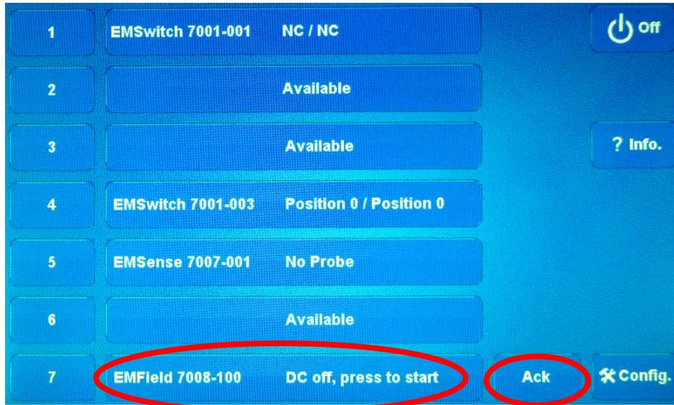
By pressing the status-button preceded by the Ack-button, the start-up procedure of the EMField will begin. Once this procedure has been completed successfully, the amplifiers in the EMField will be powered.
