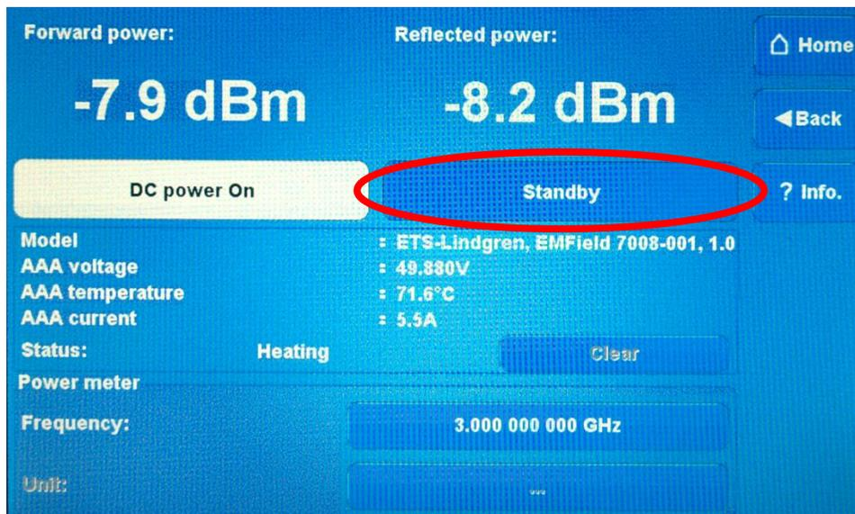
The system is now heating up to its final temperature of 75°C. It will be ready to be switched to operate once it has reached a temperature above 50°C.
