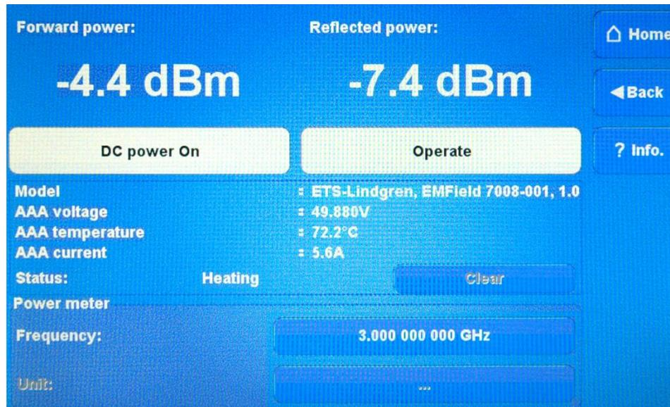
In the EMField control screen, the parameters of the system can be read. In order to generate an EM-field, the system must be switched to operate. It is important to enter the frequency of the generator driving the EMField to read the correct power meter level. Entering the actual frequency will automatically correct for the frequency dependent coupler and power meter response inside the amplifiers.
