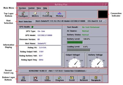
**Host Selection**: Press the combo box to select hosts that runs Bulldog Plus Service in the LAN. Users can monitor or control (need password) the UPS remotely.
