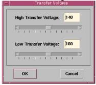
y power voltage is lower than the assigned value, the UPS will switch to backup. The output power is supplied from battery.
