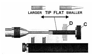
To duplicate electrode Tip Flat diameter, insert electrode into electrode wand. Extension should be beyond the desired final length.
