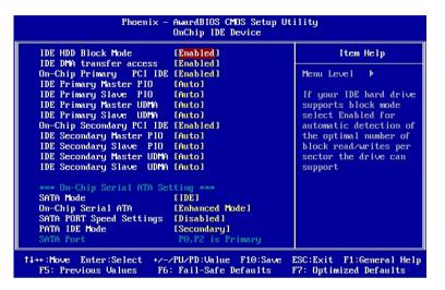
The chipset contains a PCI IDE interface with support for one IDE channel and two SATA channels. Select Enabled to activate the primary IDE interface. Select Disabled to deactivate this interface.
