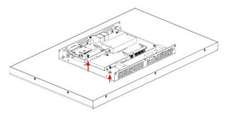
**Step 2.** Insert the HDD into the bracket and fasten 4 screws.
