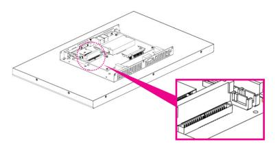
**Step 4.** By default, the SATA cables had been inserted to the according connectors. Just connect to SATA HDD with the two cables.
