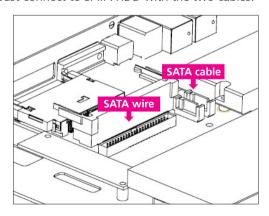
**Step 5.** Insert the HDD back and fasten 2 screws.
