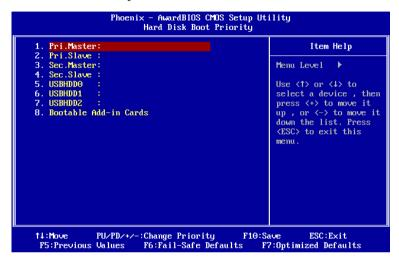
This item allows you to set the boot priority of the hard drives installed in the system.
