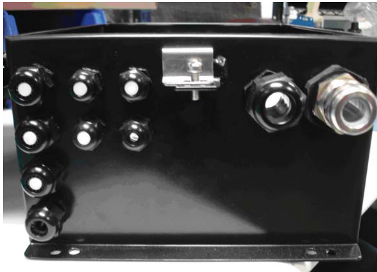
Figure 3: Cable Glands on the Bulkhead Box
