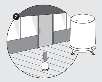
2 Find a location for the wireless rain gauge The wireless rain gauge should be placed on a flat and level surface. The location must be away from anything that may block rainfall from entering the rain collector. Rain gauge should be elevated off the ground. Placing your rain gauge on your outside deck would be an ideal location.
