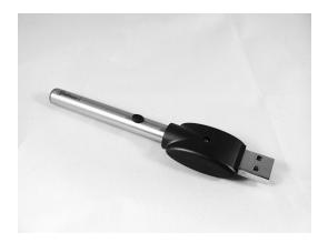
The light on the charger will blink red to let you know its working and then turn solid red while it charges. When it is finished charging the light on the charger will turn green.
