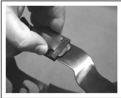
4. Squeeze together the two halves of the split location tongue on the retainer until they overlap each other. Withdraw location tongue from the gate on the headband. Repeat this operation for the opposite side.
