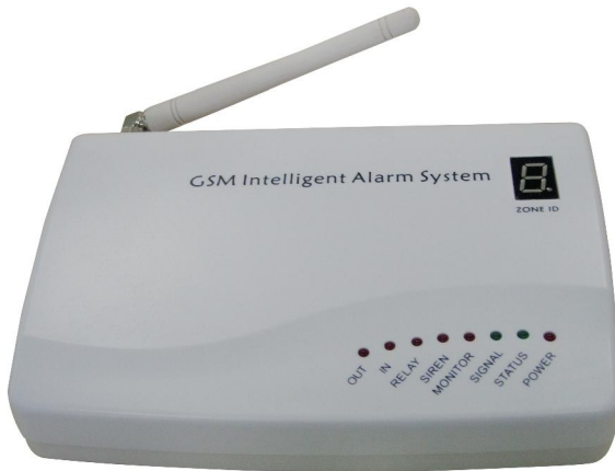
Figure1. main host of the alarm system
