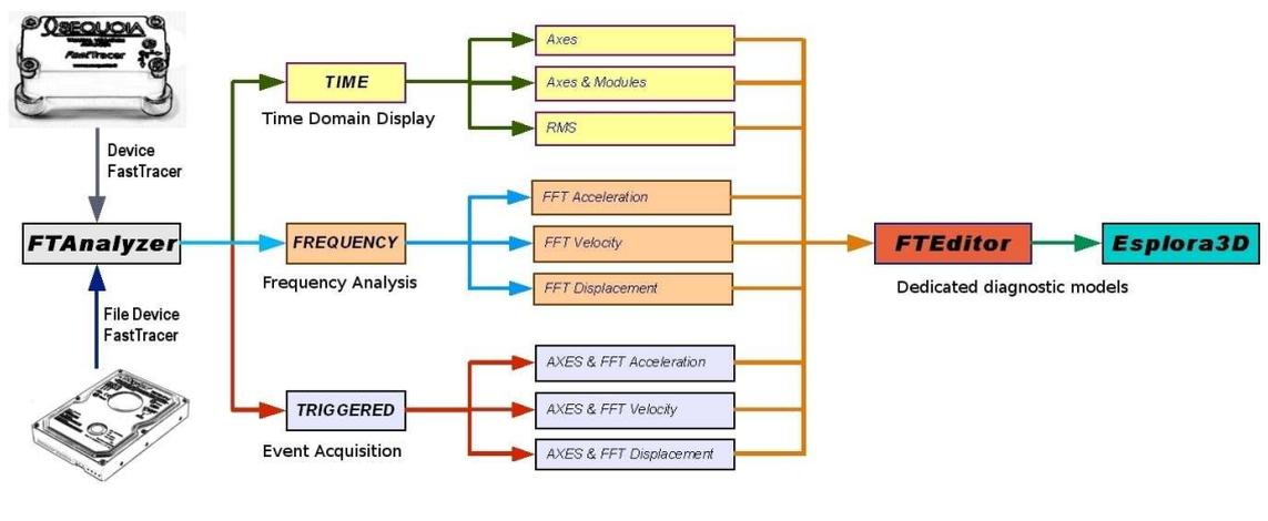
*FTAnalyzer: measurements and diagnostics*
