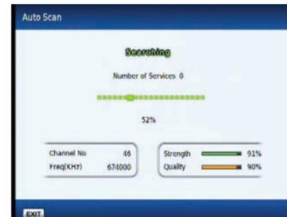
The receiver will indicate when all the Freeview channels have been successfully tuned in. Choose **OK** one or more times to progress through any remaining setup screens.
