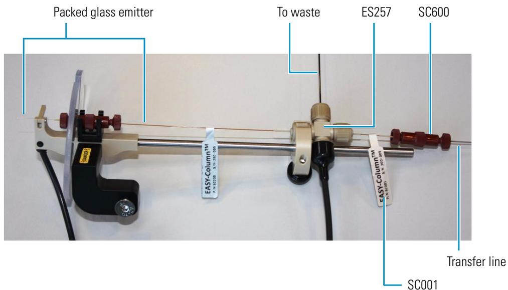
**Note** The packed glass emitter contains the stationary phase and has dual roles: as the analytical column and the emitter. The packed glass emitter is inserted through the ZDV union, which only serves as positional support.
