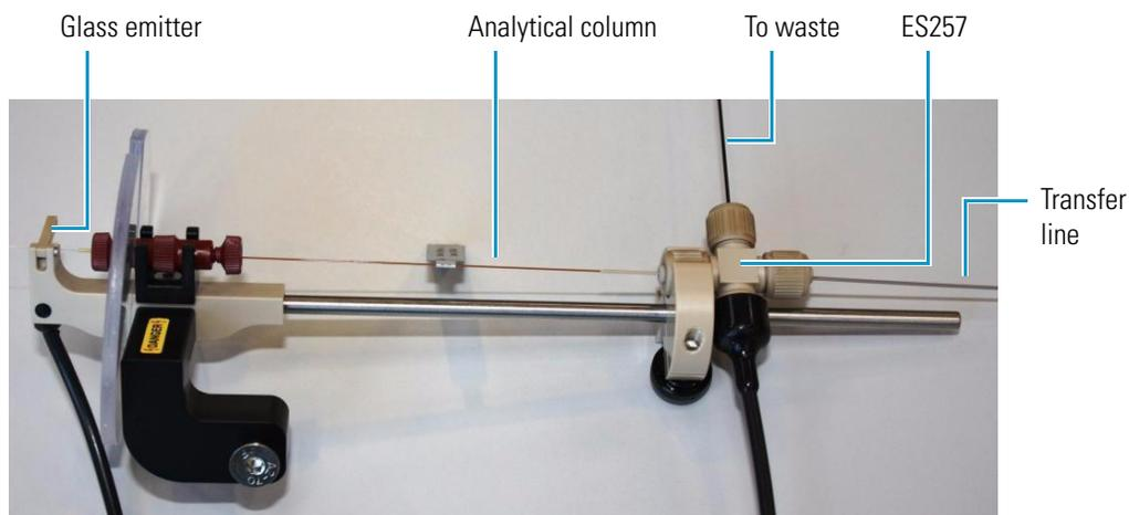
**Note** EASY-nLC software version 2.5 and later require use of the “Waste in” line connected to the vent (ES257) upstream of the analytical column in one-column configurations. For earlier software versions or with other LC systems, you can replace the Liquid Junction Cross (ES257) with a Liquid Junction Tee (ES258). Use small ID emitter tips (<math><20\ \mu\text{m}</math>) to prevent out gassing in the tip and subsequent spray instability.
