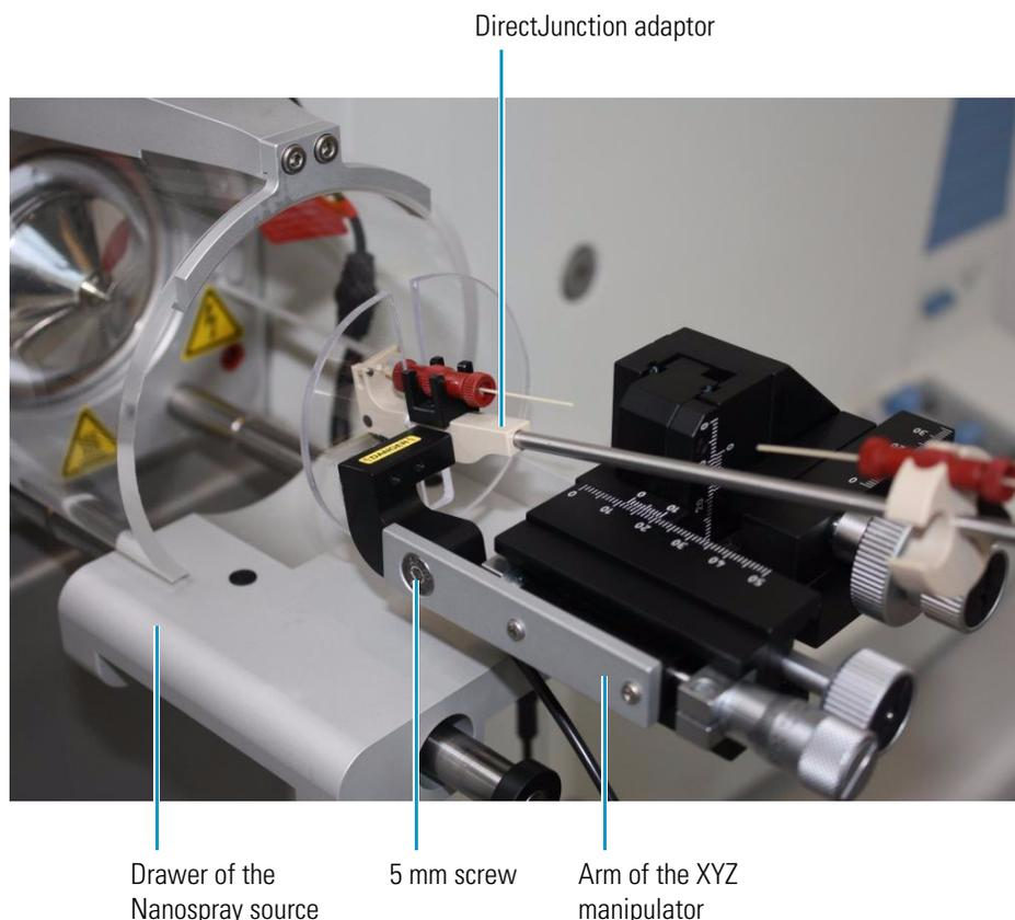
5. Use the supplied screwdriver to mount the DirectJunction adaptor on the XYZ manipulator arm. Before tightening the 5 mm screw, position the DirectJunction with the back of the DirectJunction elevated about 20° above horizontal. Tighten the screw firmly.
