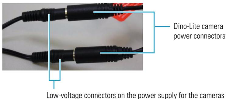
6. Connect the power adaptors for the two Dino-Lite cameras and the power adaptor for the monitor to your net power sockets.
