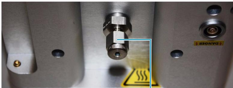
Swagelok 1/8" gas connector, option for drying- or curtain gas.
