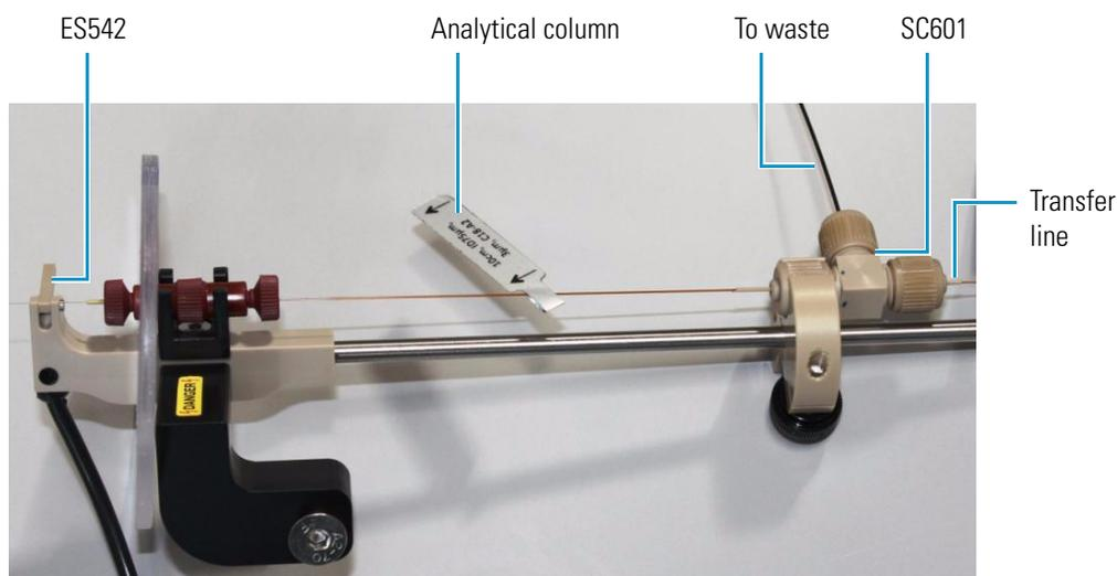
**Note** EASY-nLC software version 2.5 and later require use of the “Waste in” line connected to the vent (SC601) upstream of the analytical column in one-column configurations.
