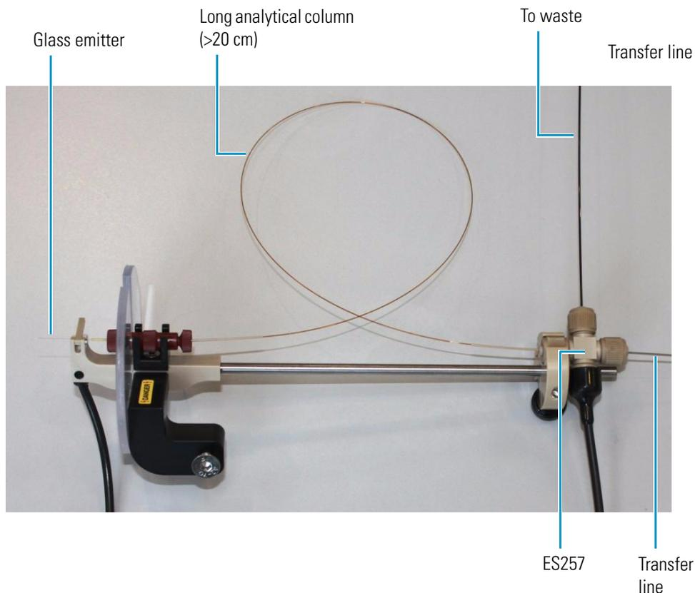
**Note** You can easily fit long columns to the DirectJunction adaptor by coiling them between the ZDV union and the vent (ES257). [Figure 27](#) shows a glass emitter and a liquid junction, but combinations with a steel emitter, a two-column configuration, or both of these are also possible.
