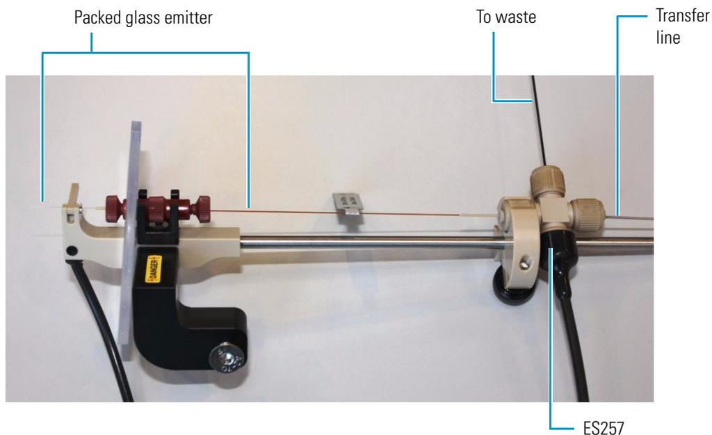
**Note** The packed glass emitter contains the stationary phase and has dual roles: as the analytical column and the emitter. The packed glass emitter is inserted through the ZDV union, which only serves as positional support.
