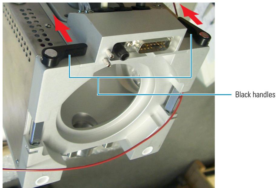
4. Take the Nanospray source and align the guiding rods of the source with the guiding holes of the mass spectrometer (see [Figure 7](#)).
