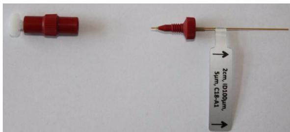
7. Tighten the nut while ensuring that the pre-column and sleeve are firmly pushed against the center of the venting tee.
