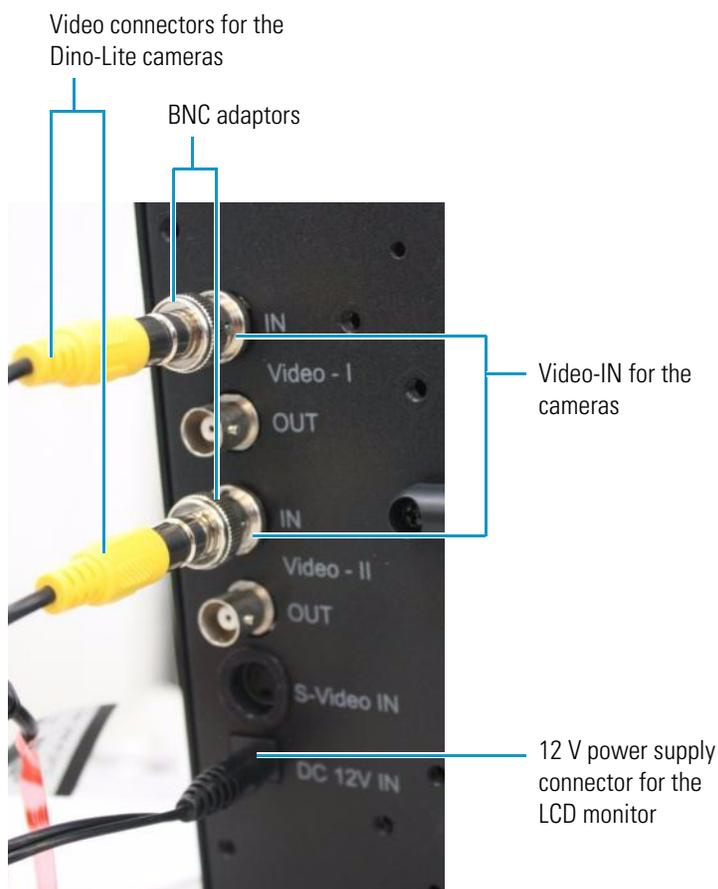
2. Connect the 12 V power supply connector to the monitor.
