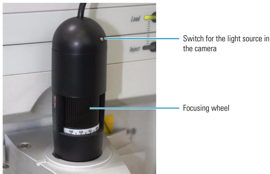
The adjustments produce a sharp image on the monitor:
