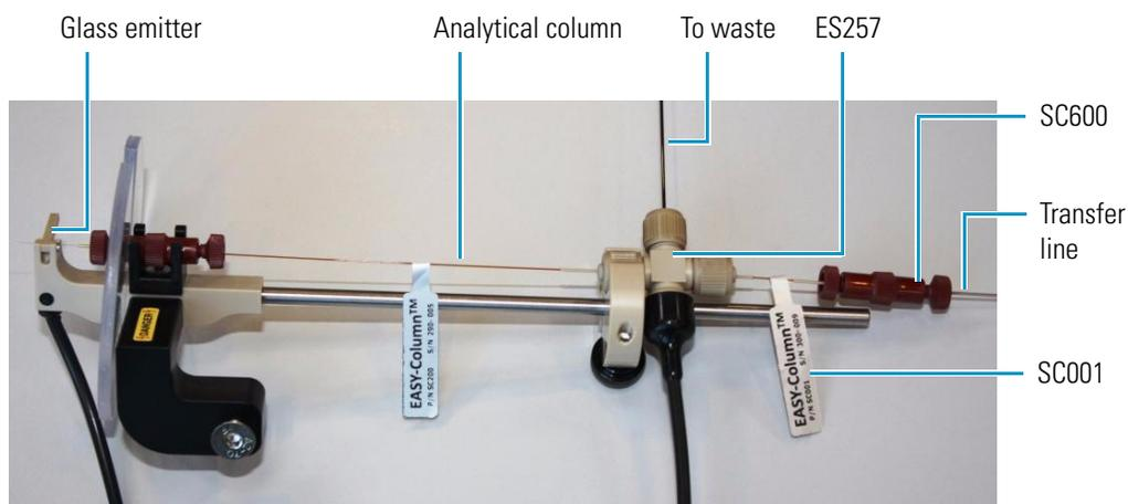
**Note** Use small ID emitter tips (<20  $\mu\text{m}$ ) to prevent out gassing in the tip and subsequent spray instability.
