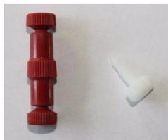
3. Insert the pre-column (SC001) through a 2 cm (0.79 in.) 1/32 in. OD sleeve (F-385) with arrows on the label pointing away from the sleeve.
