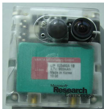
Figure 2-4: Microsoft SenseCam with transparent plastic case.
