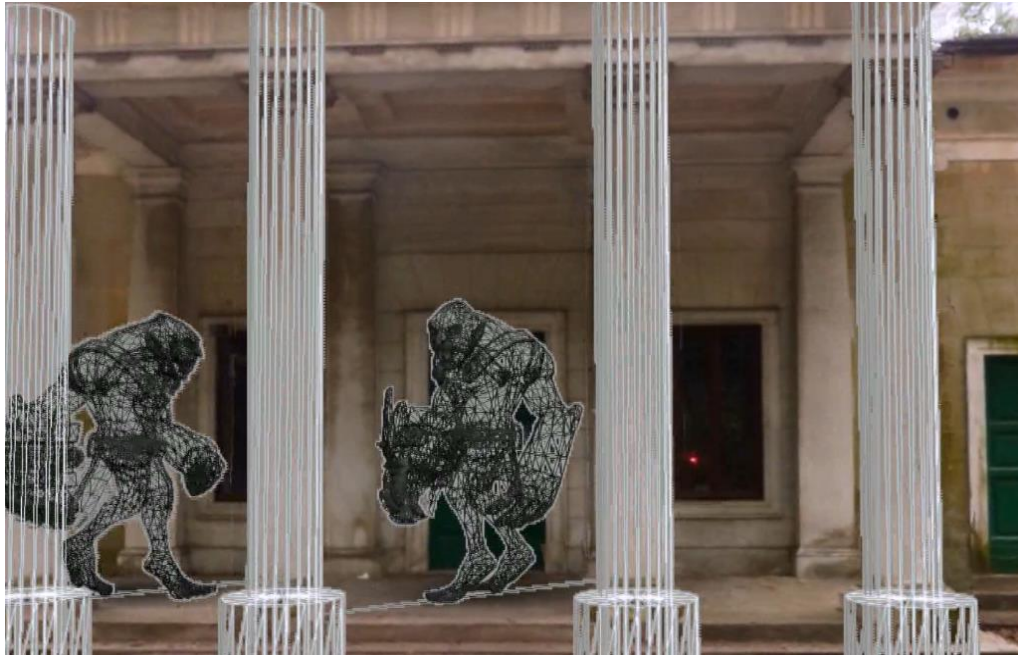
Figure 10 – The proxy-column and the 2 characters are the only 3D objects in the scene. 3D objects are placed in the space using the spatial reference provided by the point-cloud in the Unity Editor.
