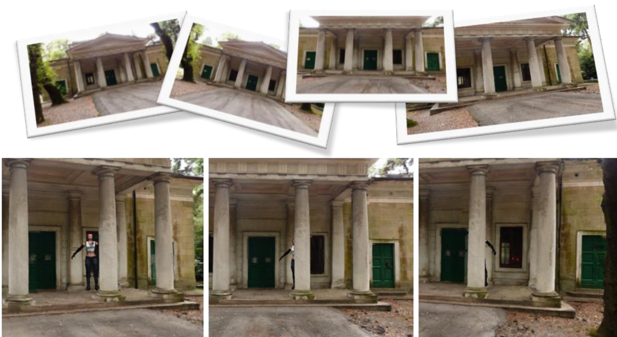
Figure 15 – Images taken during the Capture phase (above) and example of IBR scene (derived from the images) with occlusion from different views (below)
