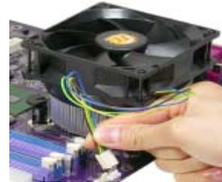
**Note 1:** To achieve better airflow rates and heat dissipation, we suggest that you use a high quality fan with 3800 rpm at least. CPU fan and heatsink installation procedures may vary with the type of CPU fan/heatsink supplied. The form and size of fan/heatsink may also vary.
