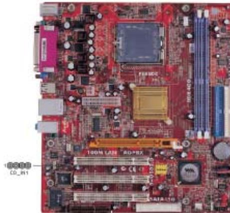
When you first start up your system, the BIOS should automatically detect your CD-ROM/DVD drive. If it doesn't, enter the Setup Utility and configure the CD-ROM/DVD drive that you have installed. On the motherboard, locate the 4-pin header **CD\_IN1**.
