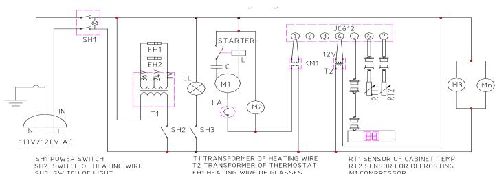
SH2 SWITCH OF HEATING WIRE SH3 SWITCH OF LIGHT JC612 THERMOSTAT EL LIGHT FA OVERLOAD PROTECTOR
