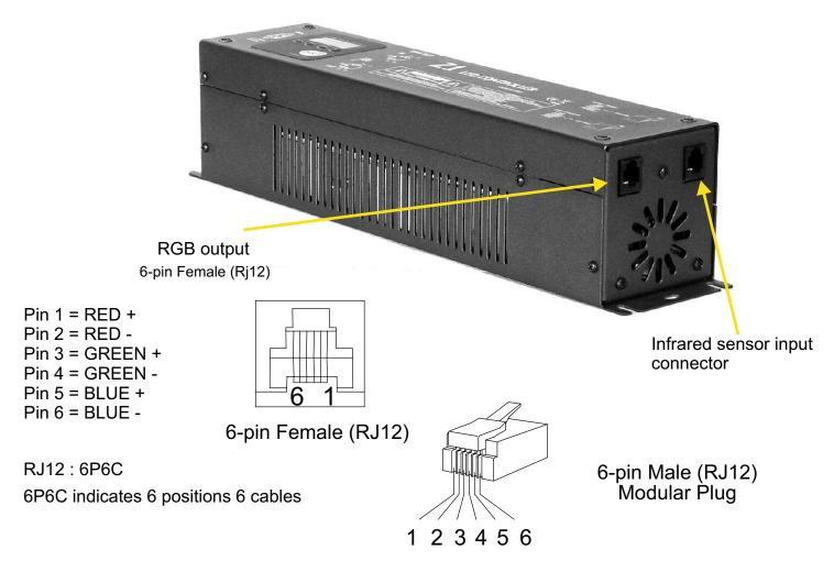
LEDs cabling connection can be done with a standard UTP TIA/EIA 568-A category 3 cable. The maximum distance between power supply and the last LED lamp in the line should not exceed 100 meters.
