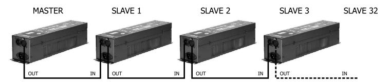
To activate Auto mode on the first unit, use the menu to run through the different modes until AUTO appears on the display, at this point press enter.
