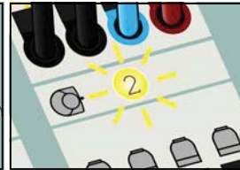
The diode of each zone lightens when the actuator opens.
