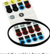
Connect the cables from the actuator with the lower row
