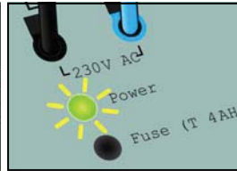
Power diode lightens up when the power is connected.
