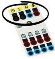
Connect the cables from the roomthermostat with the upper row
