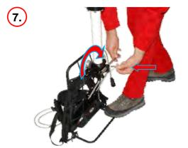
Close the locking lever and secure the locking lever with the quickpin.
