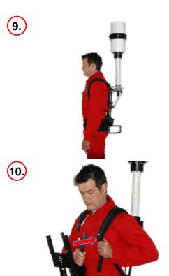
Put on the carrying frame together with the mounted AU.
