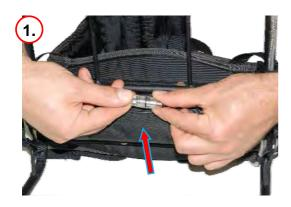
Open (screw on) the fuse holder in the DCU power cable.
