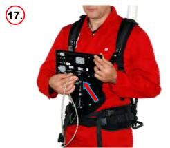
Connect the D-SUB – DCU connector for Power Supply and Audio with the DCU.
