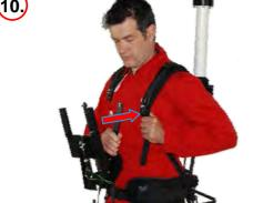
Hook up the DCU holder on the hooks located on the shoulder straps.
