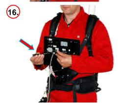
Fasten the locking screws of the D-SUB connector with the enclosed screw driver to prevent loosening and to secure watertightness of the connector.
