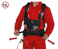
Adjust the straps of the DCU holder.
