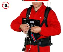
Fasten the locking screws of the D-SUB connector to prevent loosening and to secure watertightness of the connector.
