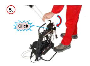
Slide the AU into the AU holder under the tilting axis. A Click is heard when the AU foot is fully engaged under the tilting axis.
