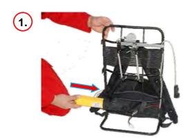
Slide the battery pack into the bag for the battery pack.
