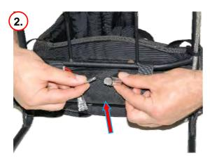
Replace the 1.6 A slow micro-fuse and close the fuse holder.
