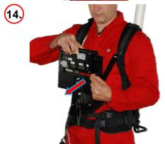
Pull the Lock pin to arrest the DCU.
