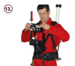
Slide the DCU into the DCU holder directed with the display to the chest.
