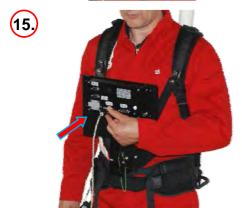
Connect the D-SUB - DCU connector for AU with the DCU.
