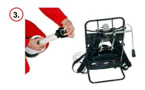
Remove the dust cap from the AU connector.
