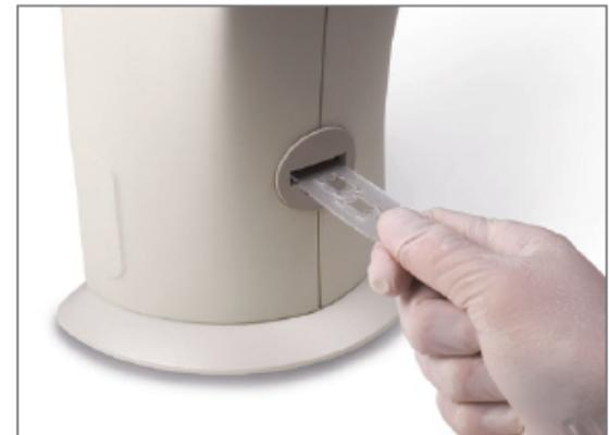
Fig. 2. Inserting the slide into the TC10 cell counter; counting automatically begins.
