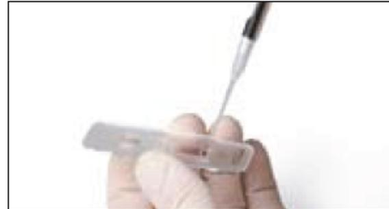
Fig. 7. Loading the TC10 counting slide.
