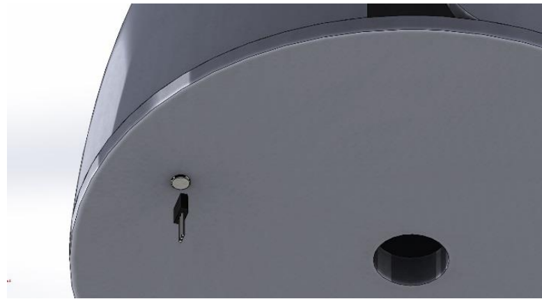
Figure 6. Correct Sensor orientation using alternate mounting method
