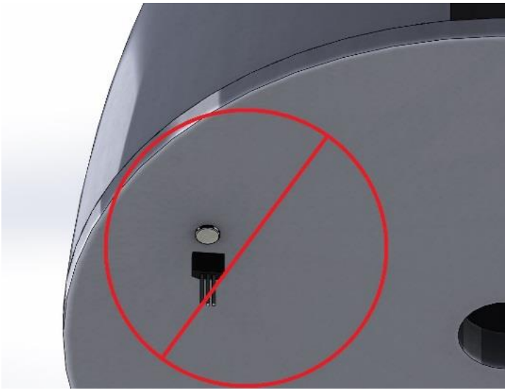
Figure 7. Incorrect orientation using alternate mounting method
