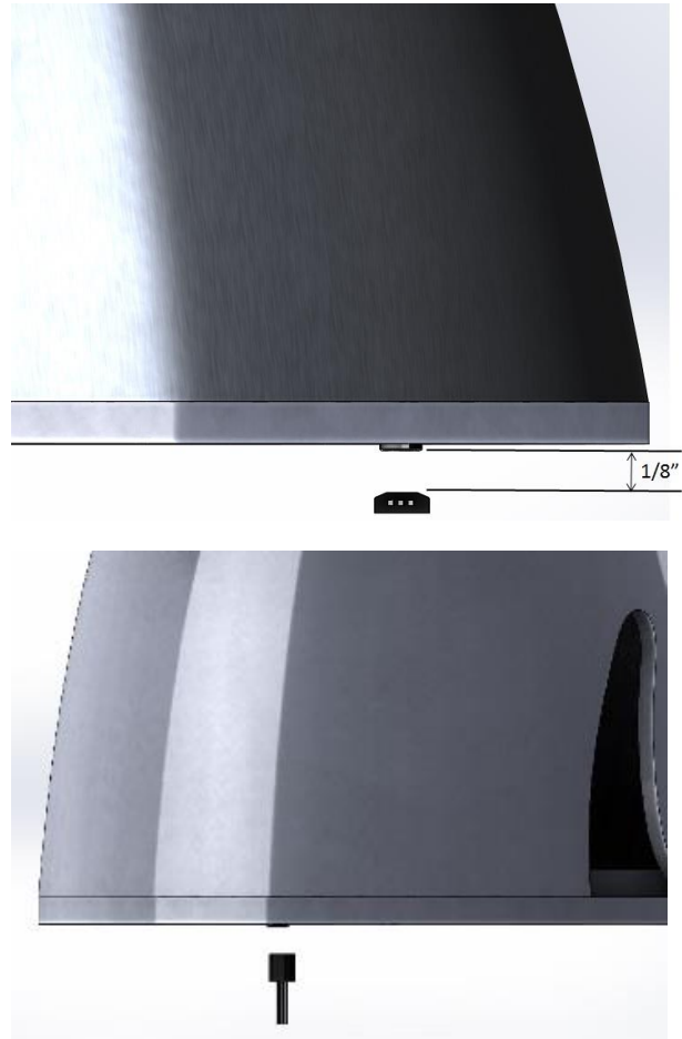
Figure 5. Mount sensor face 1/8” from magnet
