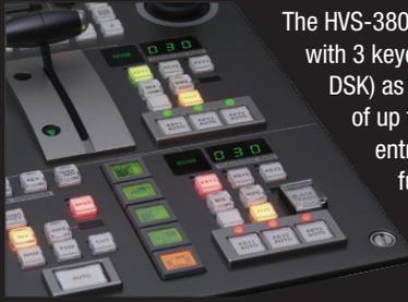
The HVS-3800HS offers a total of 6 keyers, with 3 keyers for each M/E (2 keyers + 1 DSK) as standard. This enables keying of up to 9 layers when the M/E re-entry is used. Chroma key functions are also available for KEY1 and KEY2 of each M/E. Up to 4 keyers can be used.
