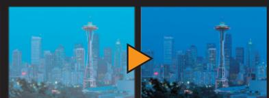
For gamma correction separately for the RGB signals in the HIGH (near 75%), MID (near 50%) or LOW (near 25%) tone.
