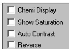
If an image will be analyzed, it is important that it not be over-saturated (too light) or under-exposed (too dark). Using **Show Saturation**, the user can see the areas of the image that are assigned to each end of the gray scale spectrum, and can adjust the imaging controls accordingly.
