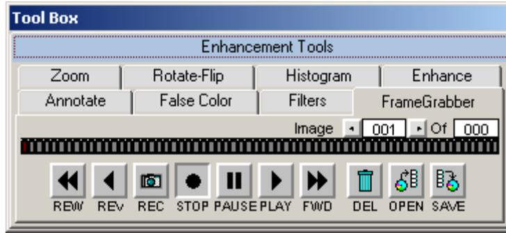
Once all images have been captured, the FrameGrabber tab will become displayed in the Tool Box. The buttons on this tab perform the following tasks:
