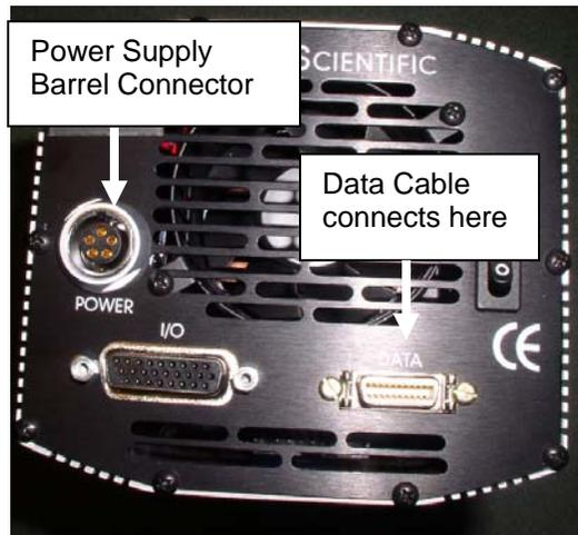
Complete the camera connection by attaching the other end of the Data Cable to the computer interface card that came preinstalled in the computer system.
