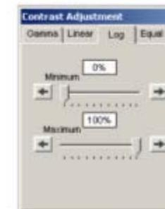
Image of film with equal Contrast Adjustment selected. Equal automatically adjusts the image display for maximum contrast which is beneficial for faint band detection.
