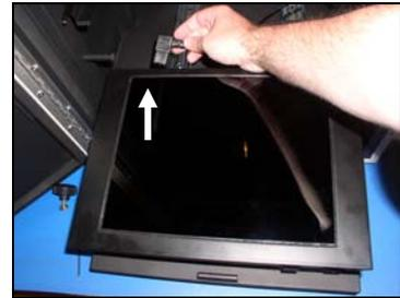
Place the UV transilluminator on the tray (making sure that its rubber "feet" are firmly seated in the holes on the tray) and then plug the cabinet's power cord into the back of the transilluminator.
