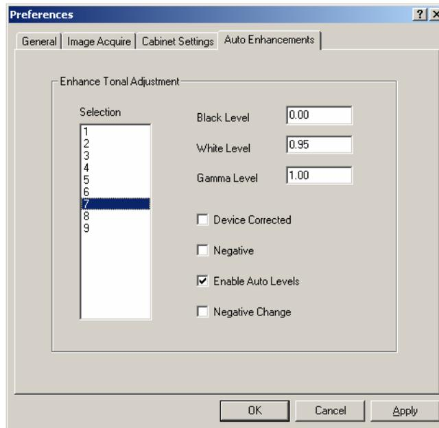
To make changes to the preferences, select your change by typing in a new value or select/de-select the appropriate box with a check mark and then select apply. Some settings may require that the software be restarted before the change will take effect.
