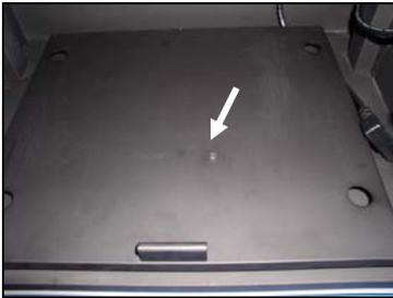
Close-up of the slide-out tray at the bottom of the cabinet. Note that there is a screw that holds the tray in place for shipping. Remove this screw to allow the tray to slide freely.
