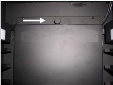
Close-up of the fold-down white light tray located at the back of the cabinet. This tray is secured by a detachable knob.
