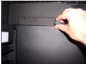
Release the white light tray by unscrewing the knob, which will allow the tray to swing down freely.
