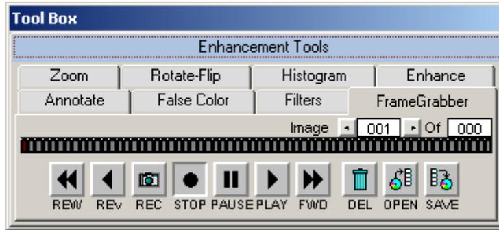
Once all images have been captured, the FrameGrabber tab will be displayed in the Tool Box. The remaining buttons will perform the following tasks:
