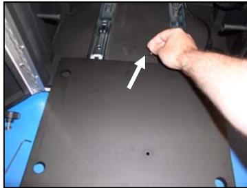
Once the tray is extended, replace the locking screw in its original position. This will prevent light from entering into the cabinet through the threaded hole.
