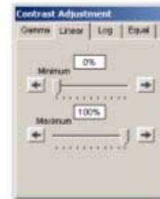
Image of film with log Contrast Adjustments selected. Log provides minimum and maximum adjustment tools from 0 to 100%. Log performs a logarithmic adjustment to the grayscale range of the displayed image.
