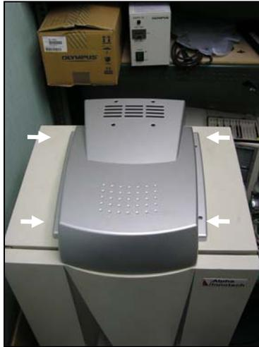
The cabinet hood is positioned over the top of the cabinet
