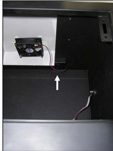
Once the hood is positioned over the top of the cabinet, plug the fan cable into the socket on the top-right side of cabinet.
