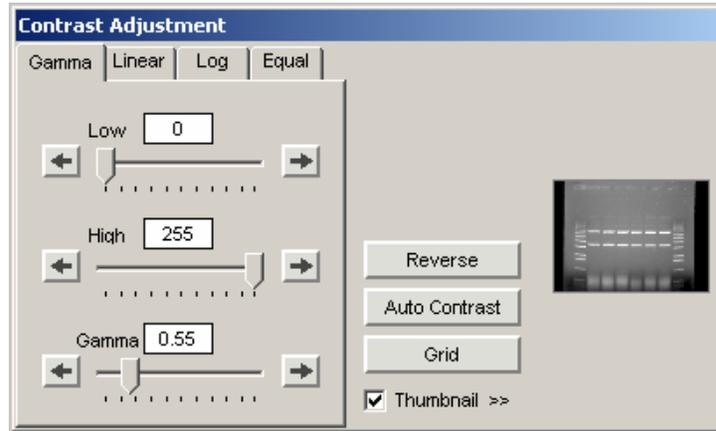
Imaging Display Tools: Black Level, White Level, Gamma Setting with B/W/G, Linear, Log, and Equalize options
