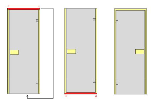
For making the door move easily, regulate the roller-lock when needed.
