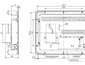
Dimensions do not include screw head Convection must be guaranteed!
