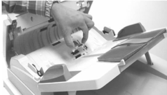
Remove the ADF pad in this direction.
