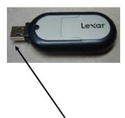
This end goes in the USB port on your computer (you will need to remove the protective cap on the end
