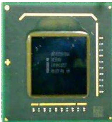
The Intel® System Controller Hub US15W is a low-power chipset in one small 22x22mm package. It combines the Intel® Graphics Media Accelerator 500, memory controller, and I/O controller in a single-chip solution while featuring advanced 3D graphics and extensive I/O capabilities such as USB2.0, SDIO and PCI Express. It supports Intel® High Definition Audio and hardware video decode acceleration, a 400/533 MHz CMOS front-side bus, dual independent display.
