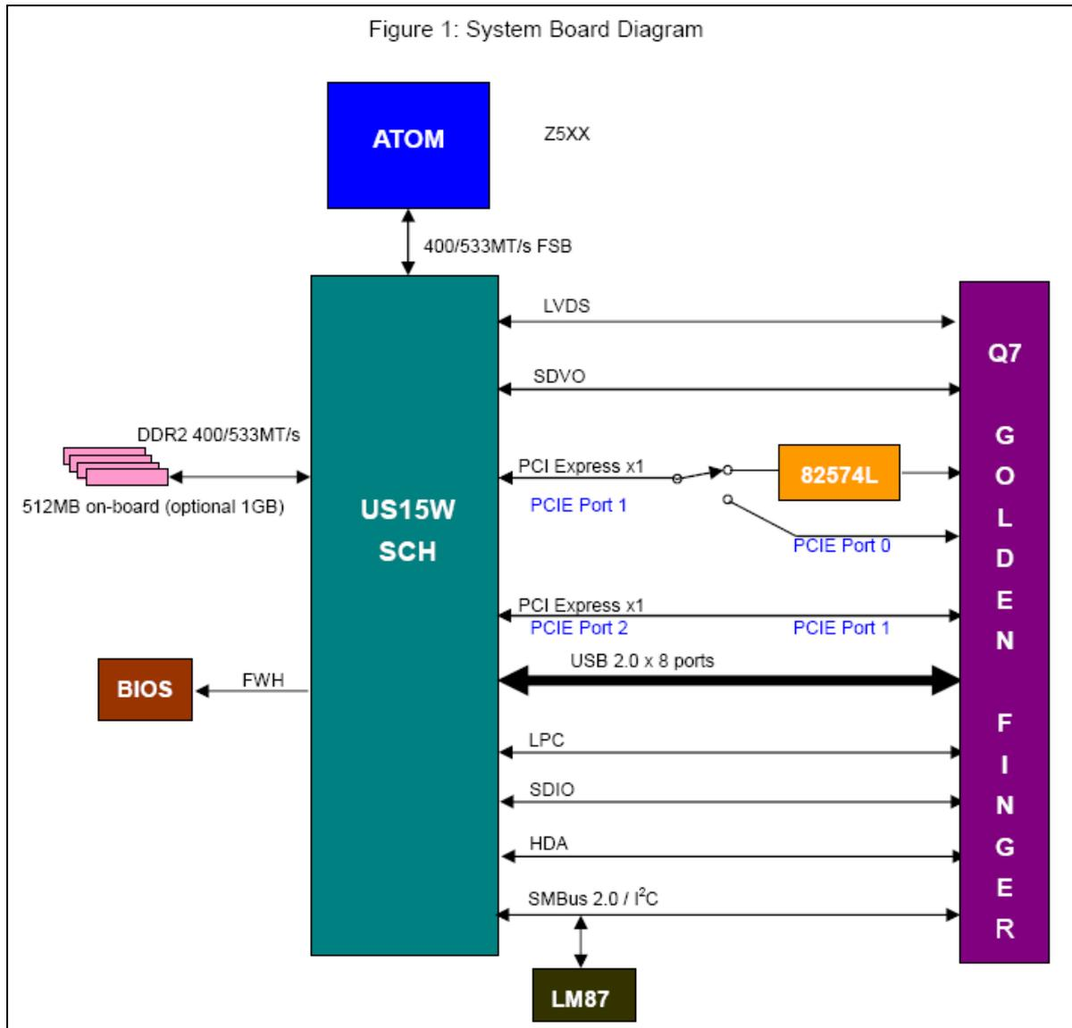
PQ7-M100G Series System Block Diagram
