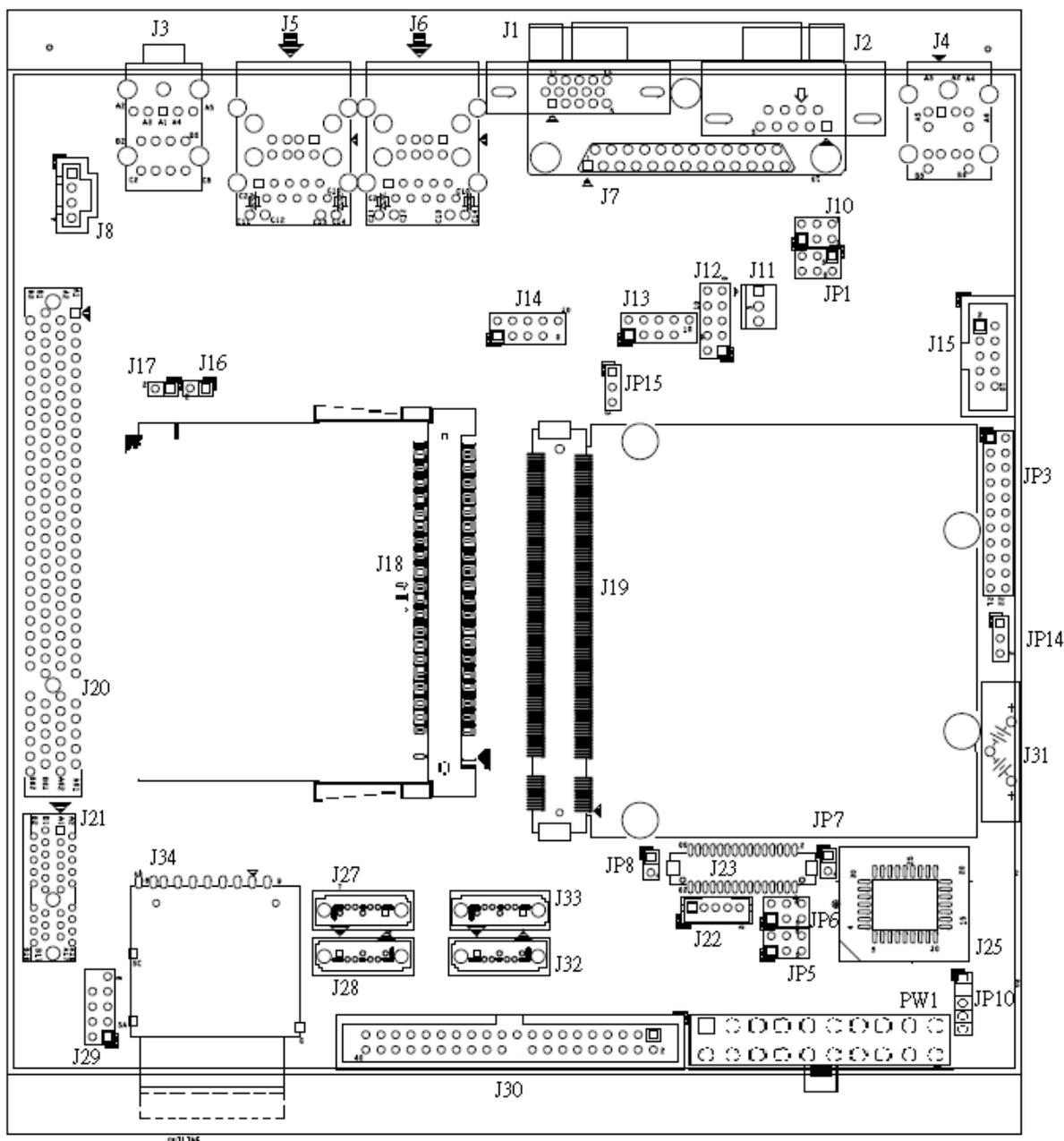
Figure 2-1 PQ7-C200 Jumper & Connector Location
