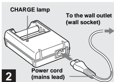
**➔ Connect the battery charger to a wall outlet (wall socket) using the power cord (mains lead).**
