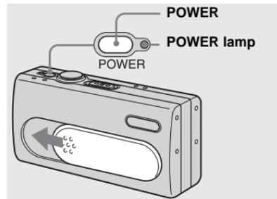
➔ Slide the lens cover in the direction of the arrow or press **POWER**.
