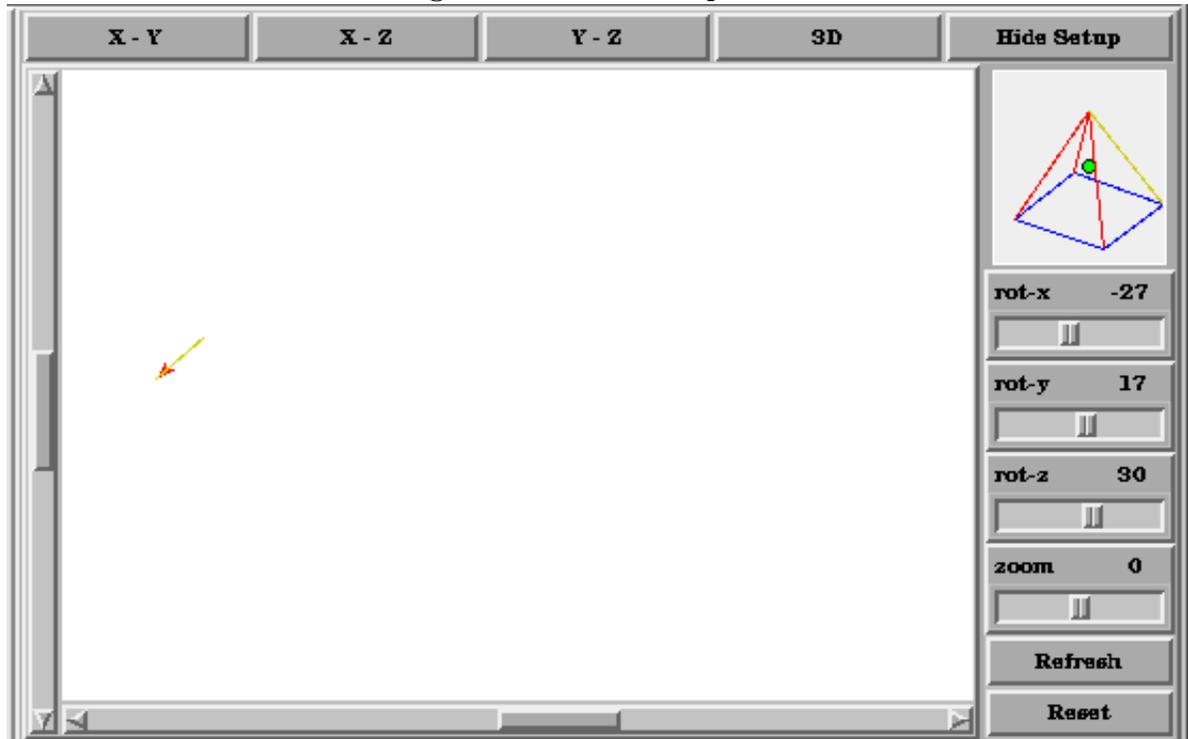
Backplot [Backplot] will show the tool path that can be viewed from a chosen direction. '3-D' is the default. Other choices and controls are displayed along the top and right side of the pop-in. If you are in the middle of a cut when you press one of these control buttons the machine will pause long enough to re-compute the view.
