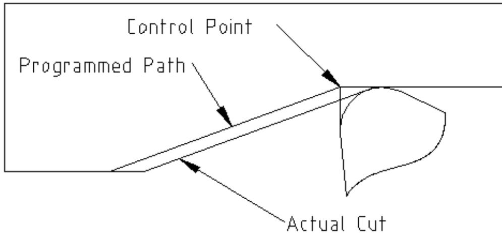
In the above example it is a simple exercise to adjust the programmed path to give the desired actual path by moving the programmed path for the ramp to the left the radius of the tool tip.
