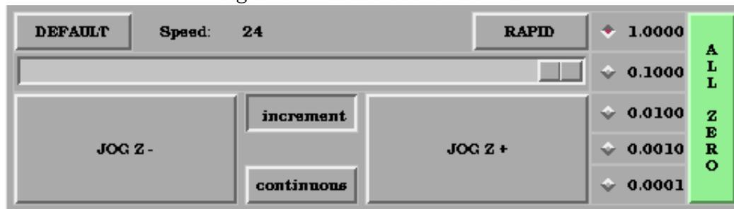
A button has been added to designate the present position as the home position. We felt that a machine of this type (Sherline 5400) would be simpler to operate if it didn't use a machine home position. This button will zero out any offsets and will home all axes right where they are.
