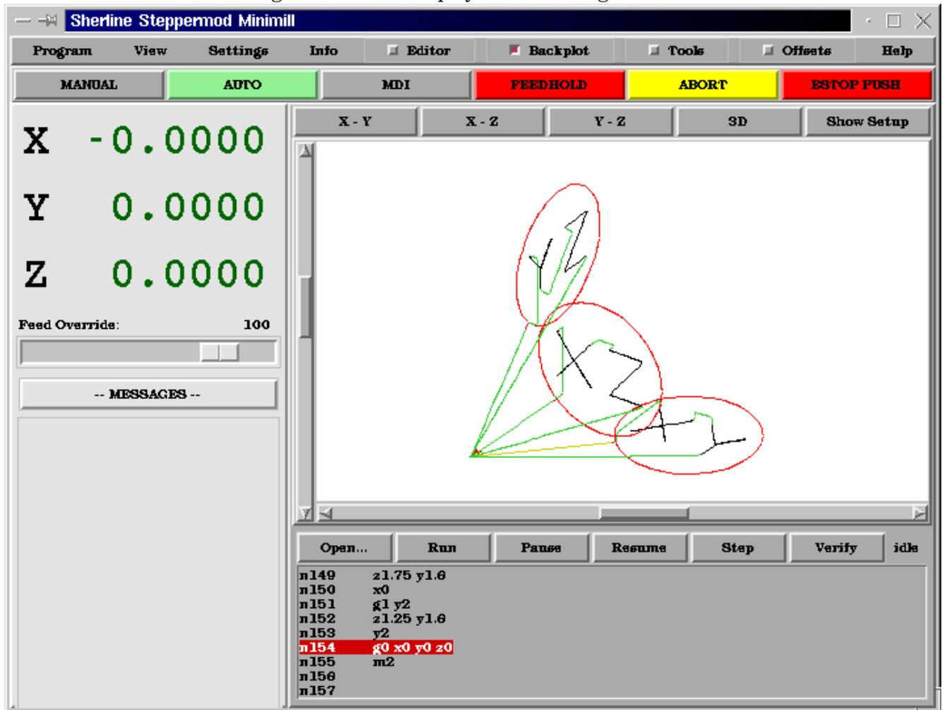
The Mini screen is laid out in several sections. (See Figure8.1 ) These include a menu across the top, a set of main control buttons just below the menu and two rather large columns of information that show the state of your machine and allow you to enter commands or programs.
