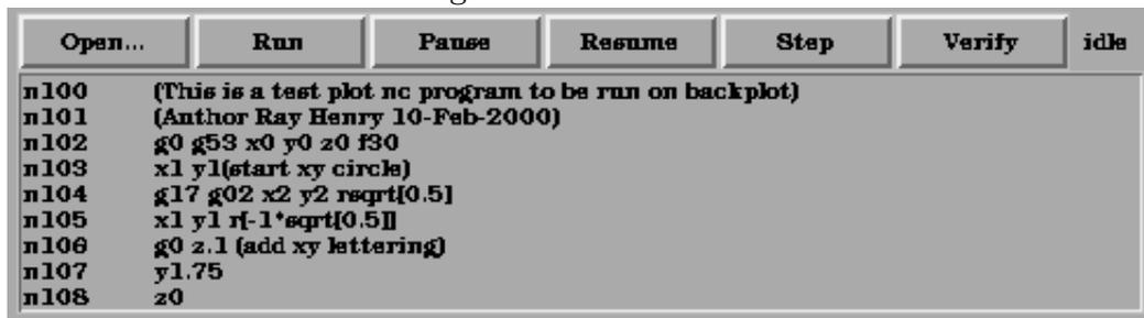
Auto mode does not normally display the active or modal codes. If the operator wishes to check these, use menu Info -> Active\_G-Codes. This will write all modal codes onto the message scratch pad.
