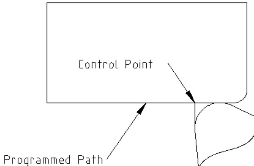
In this next figure you can see as the tool approaches the end of the part the control point still follows the path but the tool tip has left the part and is cutting air. You can also see that even though a radius has been programmed the part will actually end up with a square corner.
