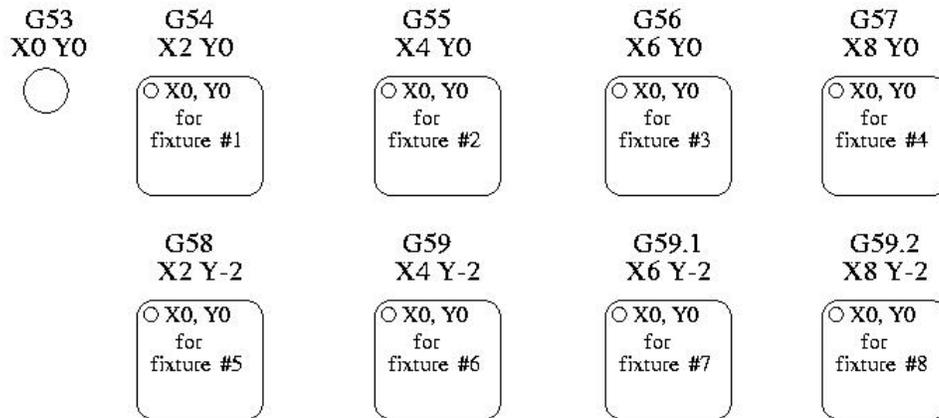
Figure 13.1: Fixture Offsets
