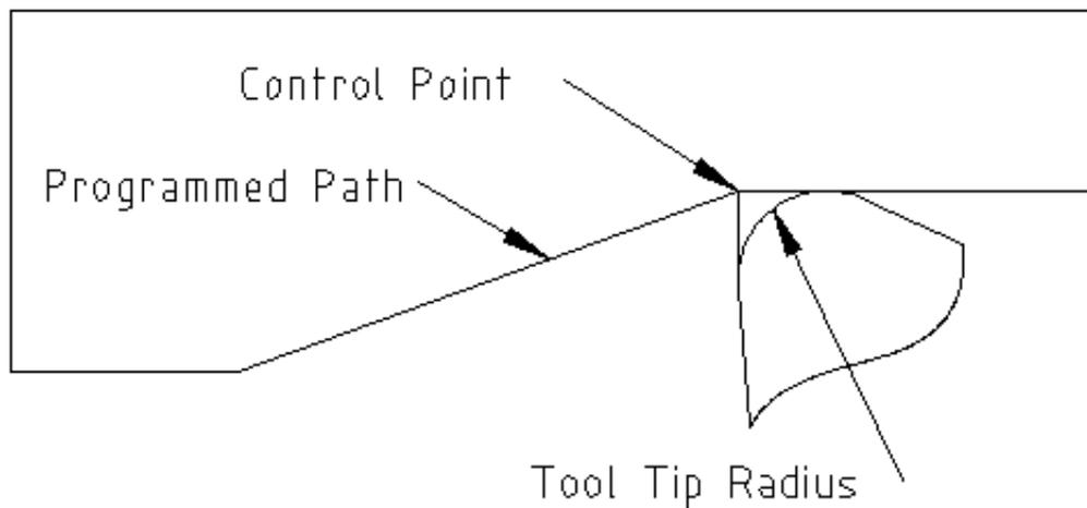
Now as the control point progresses along the programmed path the actual cutter edge does not follow the programmed path as shown in the following figure. There are two ways to solve this, cutter comp and adjusting your programmed path to compensate for tip radius.
