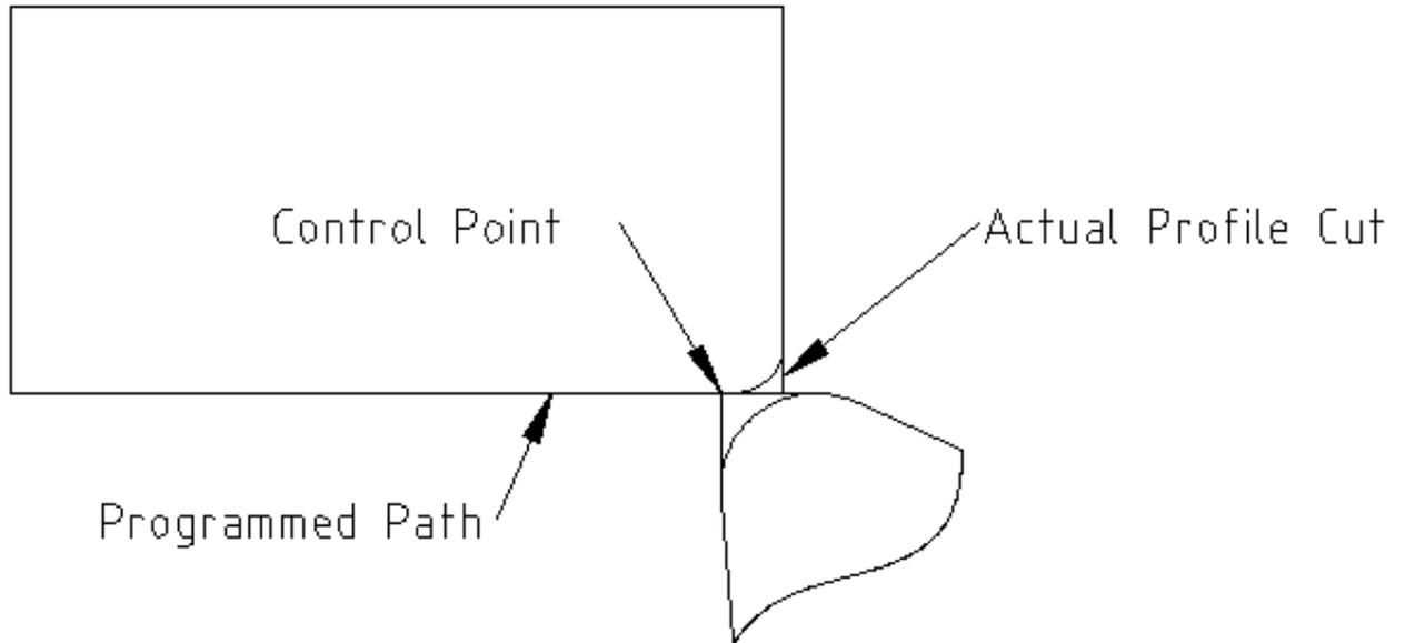
Now you can see as the control point follows the radius programmed the tool tip has left the part and is now cutting air.
