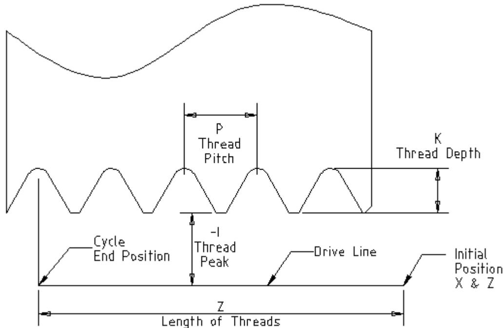
**Drive Line** A line through the initial X position parallel to the Z.
