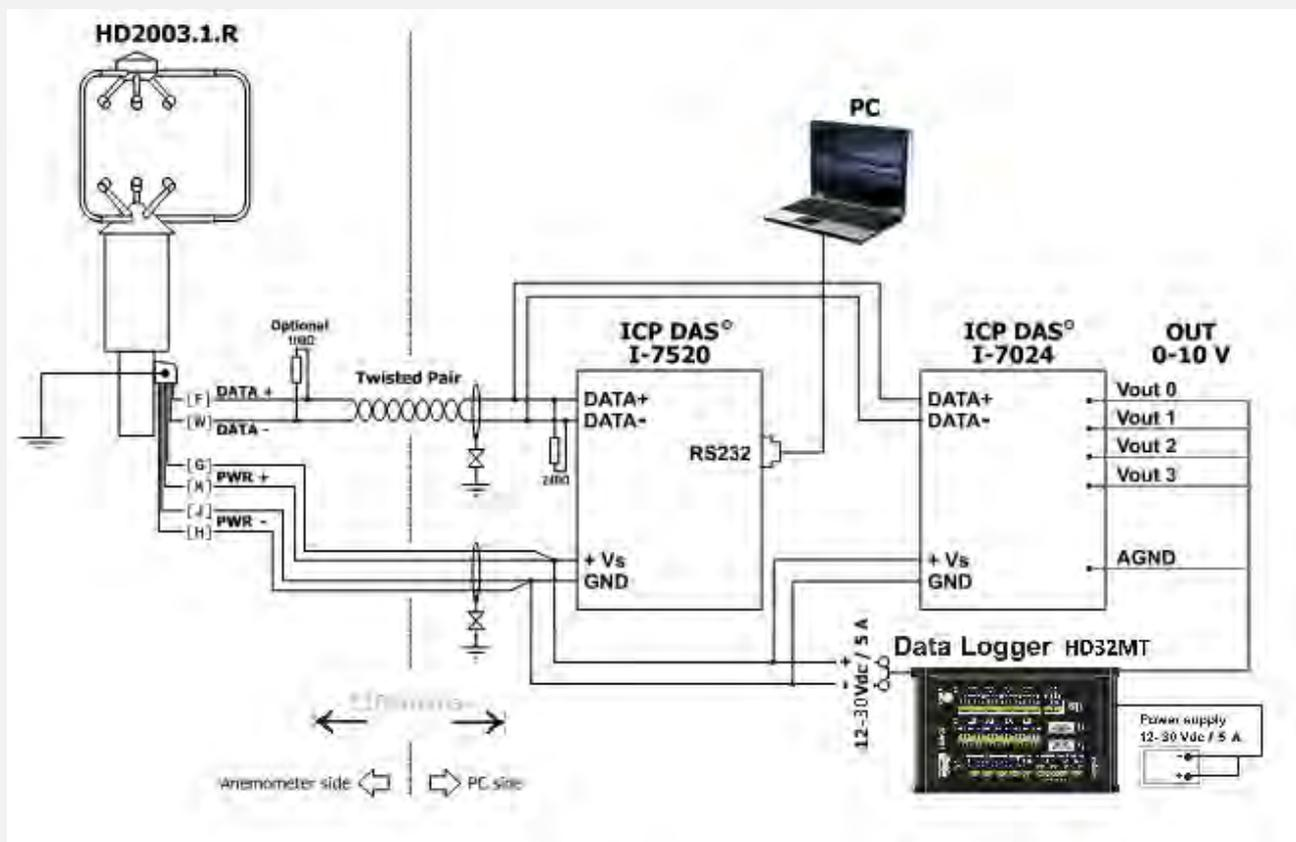
The Host computer is used only to configure the ICP DAS I-7024 ® modules and the Anemometer, or for debug. The Analog Outputs of the module, converge for storage in the datalogger *DeltaOhm HD32MT.1*, placed close to the module. The journey of analog signals is very short, so it is not affected by electromagnetic interferences.
