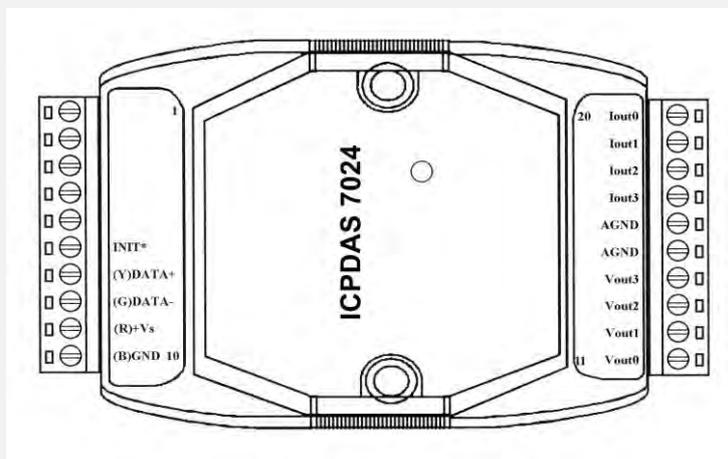
Remote interface module ICP DAS I-7024 ®
