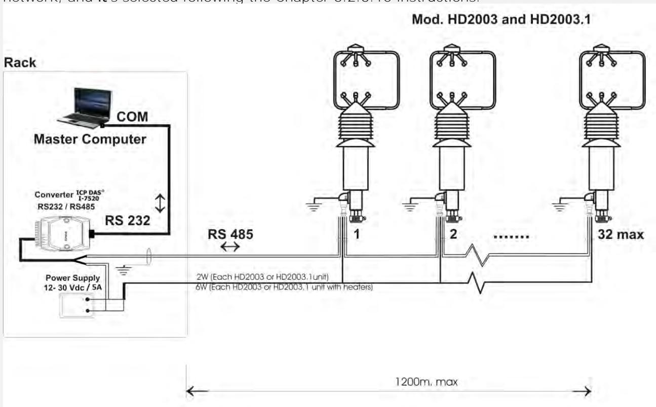
Connect the Anemometers in the RS485 Multidrop network and set electrical connections as illustrated in Chapters 2.4.1 and 2.4.3. After the power is supplied, each HD2003 unit (*Slave*) will work on **Stand by** continuing to execute its normal measurement cycle, waiting for commands from the Computer Host (*Master*).
