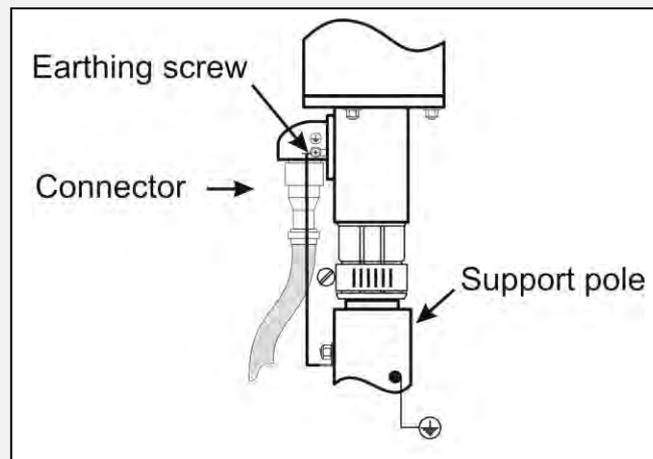
The connection in the figure was performed by using a screw on the support pole. It's also possible to make the connection by using a cable tie around the support pole.
