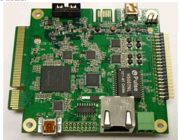
3"x3" low-power modem development board
