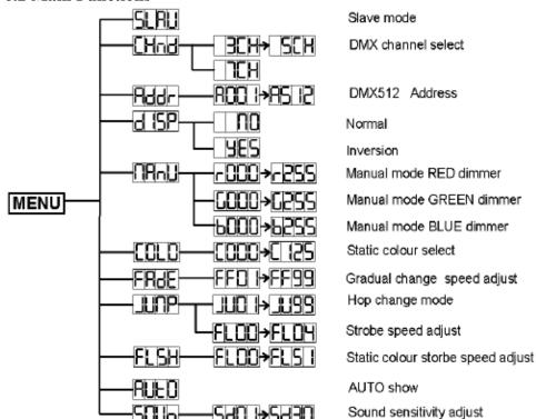
Your Talent Sound & Lighting fixture may be operated as a stand-alone device that runs on pre-programmed routines or sound activation, in master/slave mode with other devices, or via an external DMX512 controller. In DMX mode it is configurable to be controlled by 3, 5, or 7 channels.
