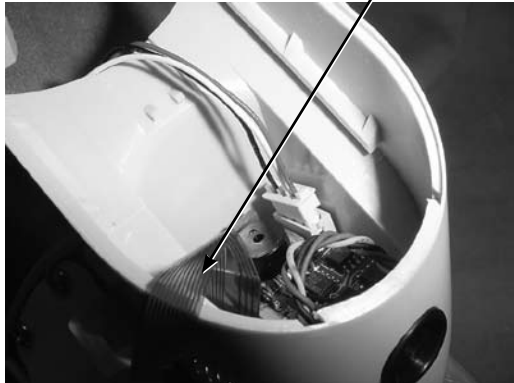
Figure F.3.2g: Unclasp Battery Connector
