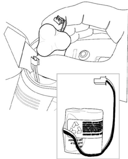
Figure F.3.1Ac: Routing battery wires
