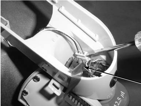
Figure F.3.2f: Lift Battery Connector
