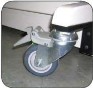
LOCK To lock, push locking tab down.
