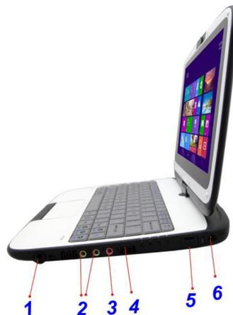
1. **Stylus Pen Slot** – the stylus pen for the touch screen is stored here.
