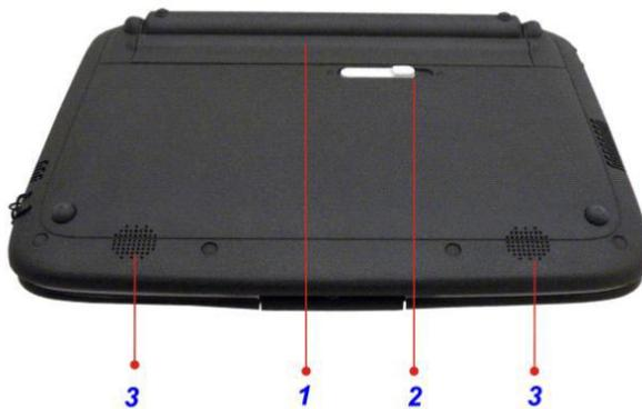
1. **Battery Bay** – this compartment contains the battery pack for your system.
