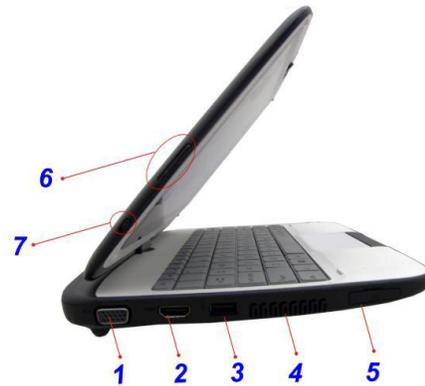
1. **External Monitor Port** – use this port to connect to an external monitor.
