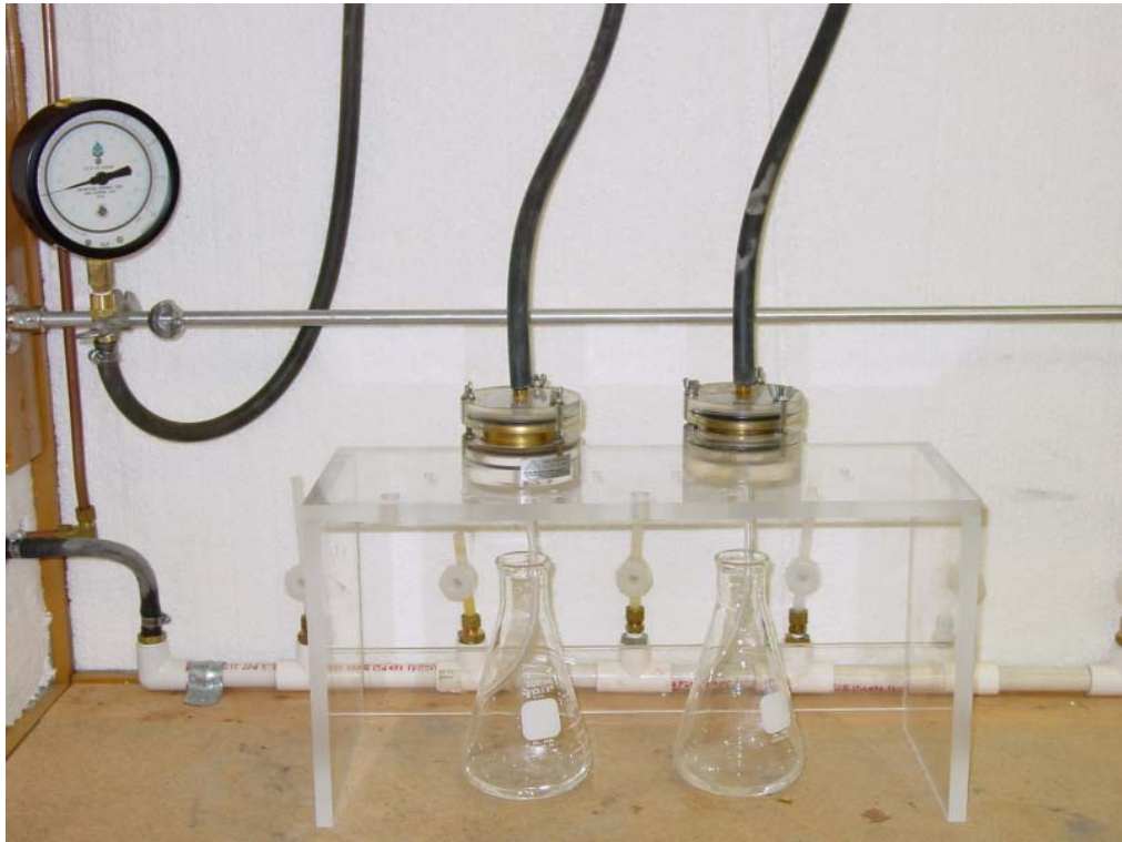
Fig.3: Tempe cells connected to pressure lines and outflow flasks.
