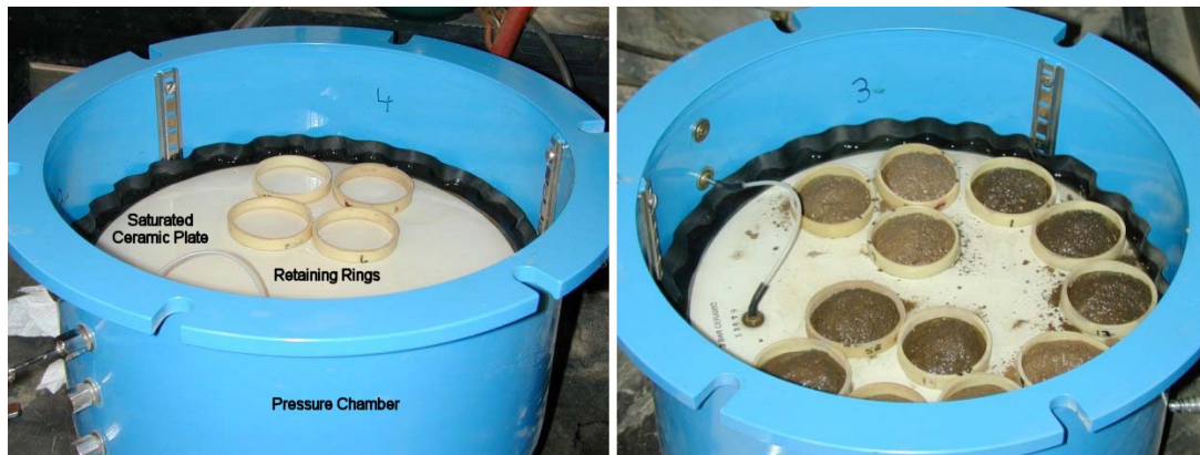
Fig.4: Pressure chamber with saturated ceramic plate and retaining rings.
