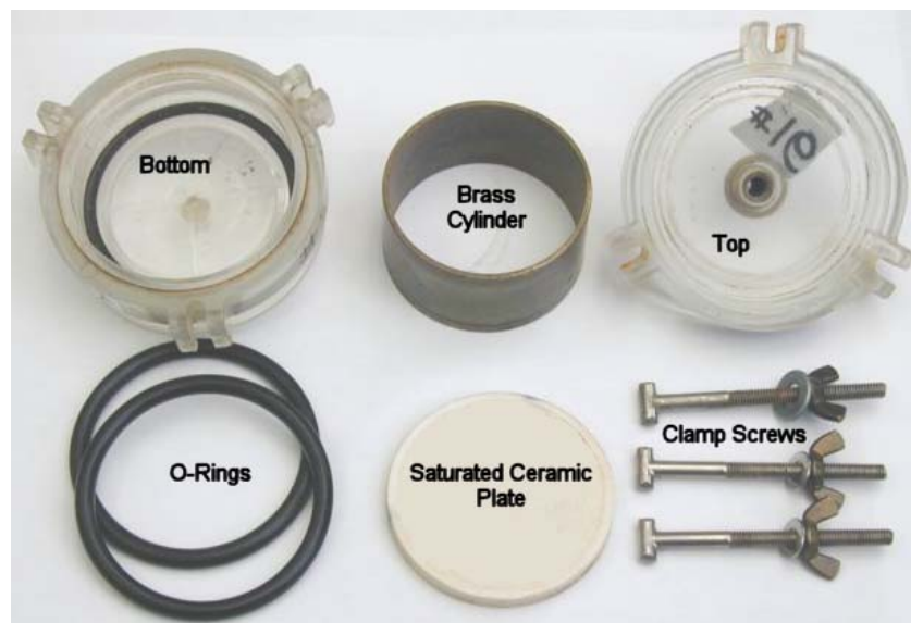
Fig.1: Tempe cell parts
