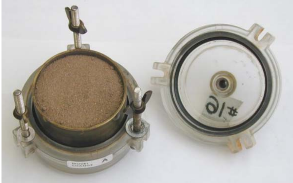
Fig.2: Assembled Tempe cell with sample
