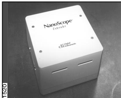
**Figure 230-2 Extender™ Electronics Module—required for frequency phase detection MFM and EFM.**
