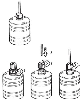
**Fig 2.** Connection of 1/16" tubing to the flow cell.
