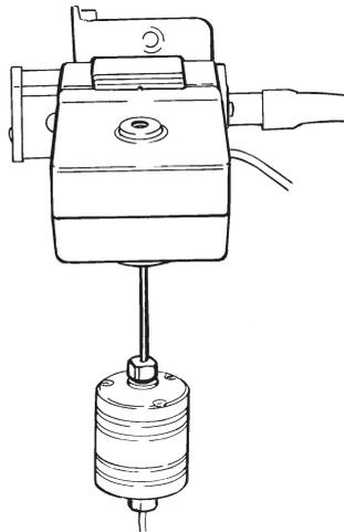
**Fig 1.** Connection of the gradient monitor flow cell.
