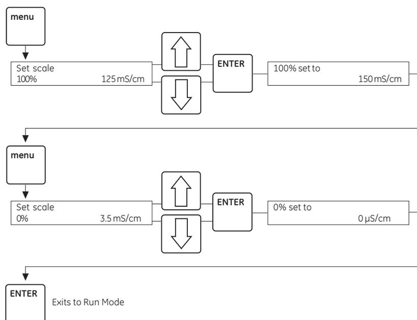
**Fig 14.** Fixed scale setting.
