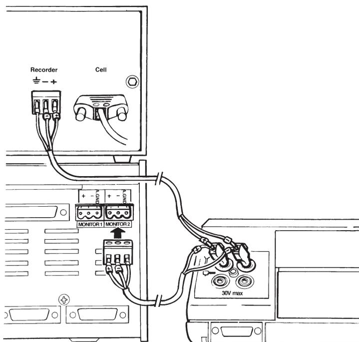
**Fig 5.** Connection of the gradient signal to LCC-501 Plus and to the recorder.
