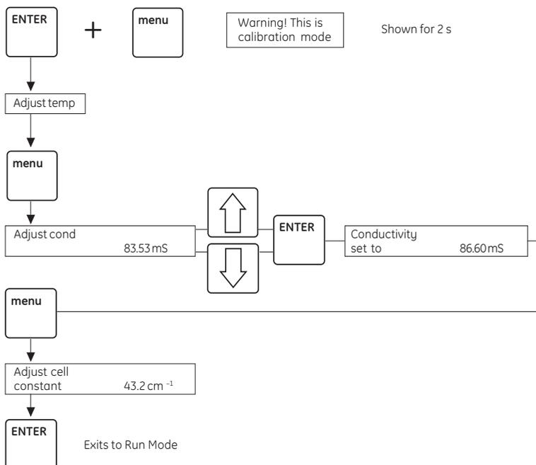
**Fig 19.** Calibration of cell constant.
