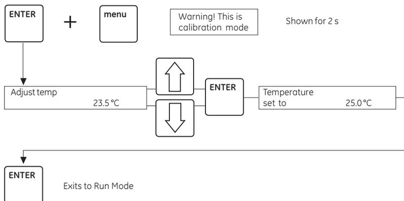
**Fig 18.** Calibration of the temperature sensor.
