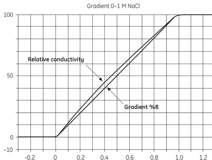
Fig 10. A typical conductivity gradient.
