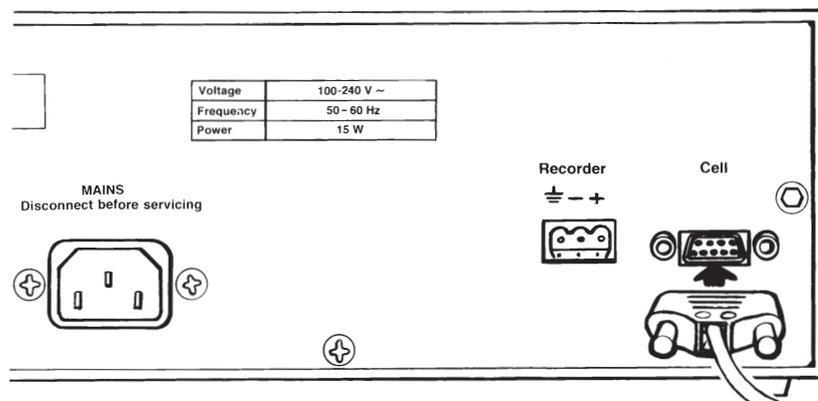
Fig 3. Connection of flow cell.
