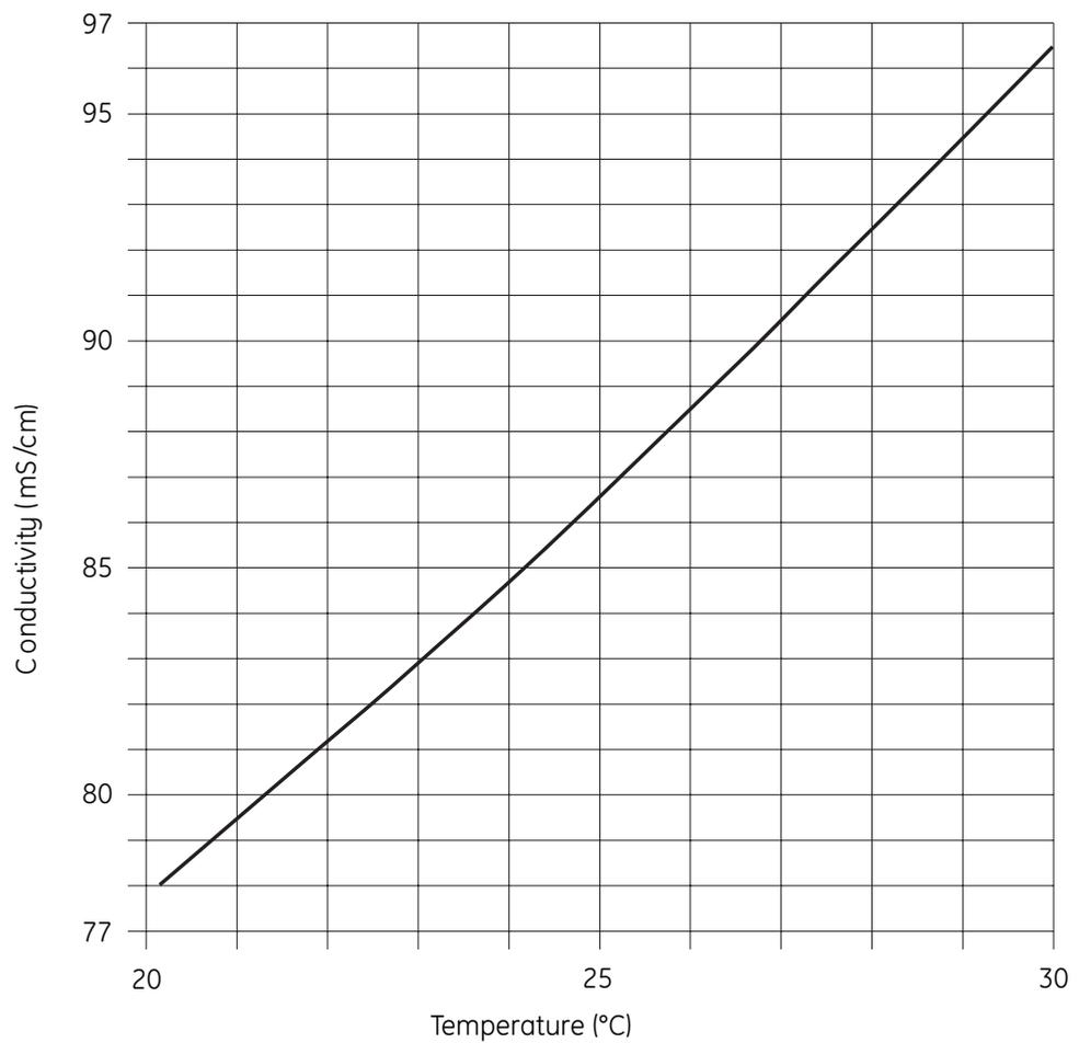
**Fig 20.** Conductivity of 1 M NaCl at 20–30 °C.
