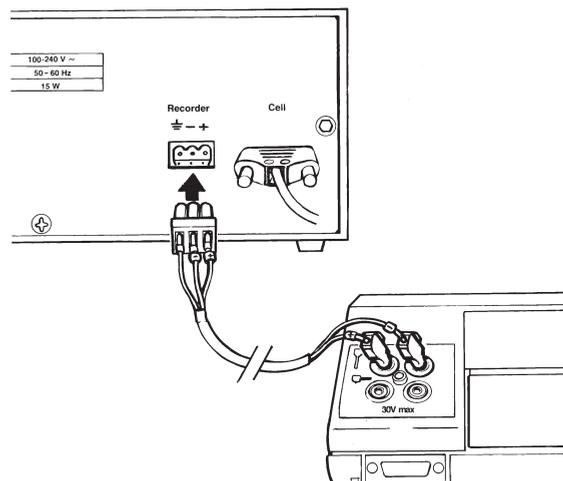
Fig 4. Connection of the recorder.
