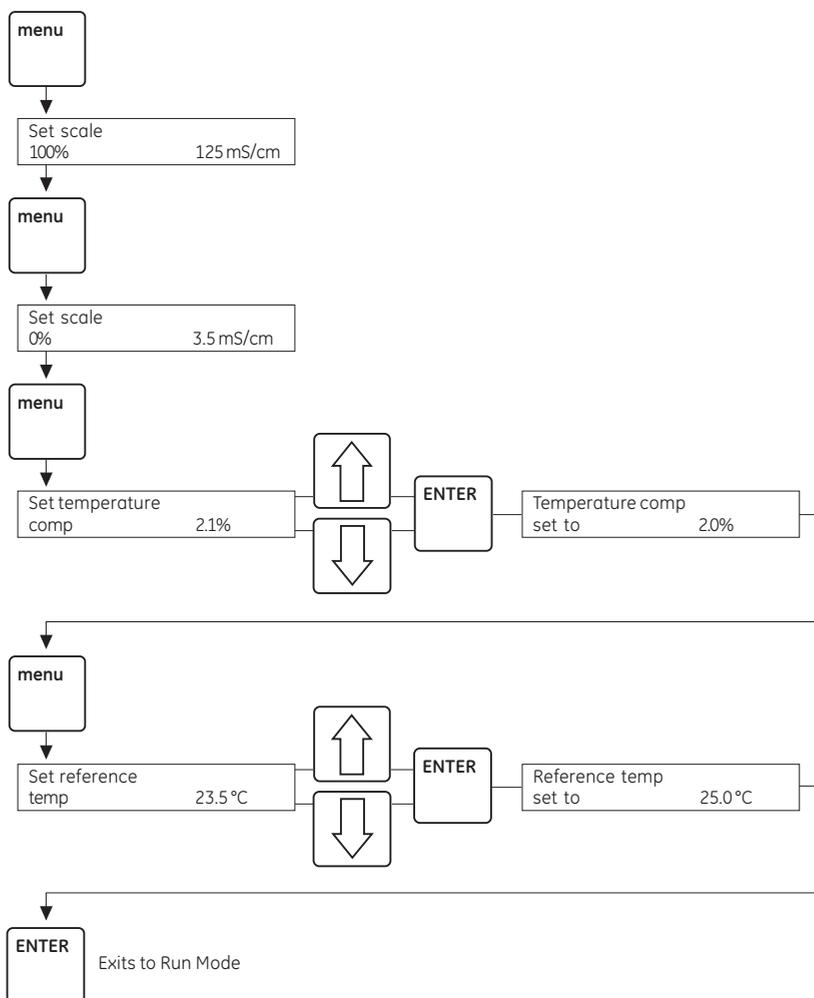
**Fig 15.** Temperature compensation setting.
