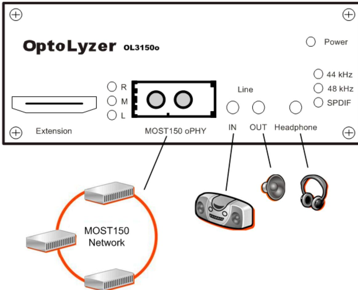
Figure 3-1: Connectivity Diagram—Front Panel
