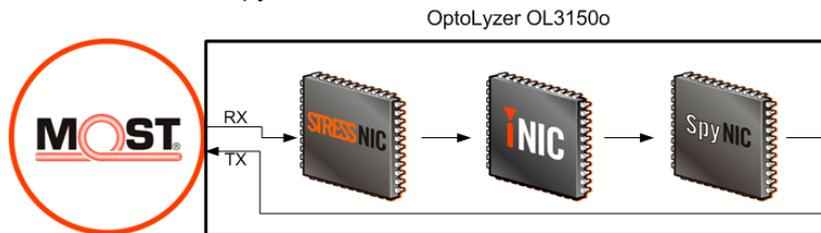
Figure 2-3: Order of Chips inside the OptoLyzor OL3150o - Old Design
