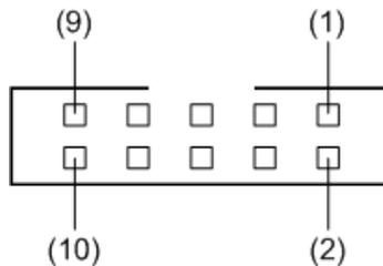
Figure 6-2: Trigger Interface Front View
