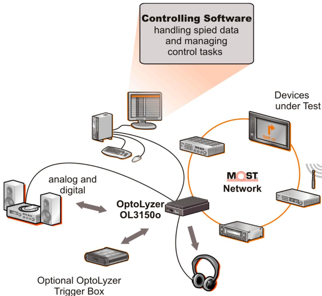
Figure 2-1: Possible Scenario of an OptoLyzer OL3150o
