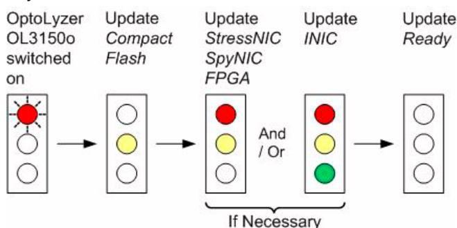
Figure 4-1: Automatical Update Procedure
