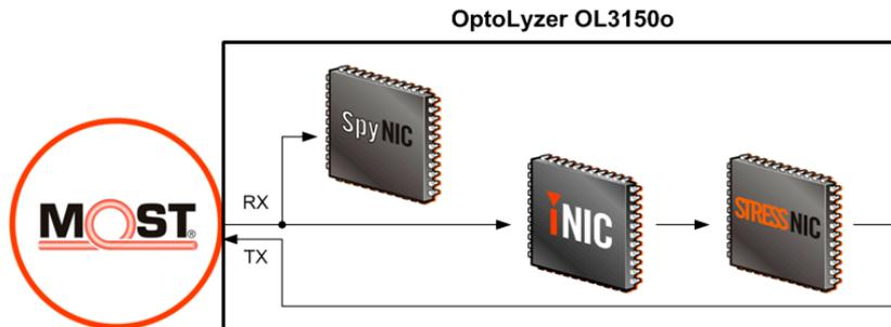
Figure 2-2: Order of Chips inside the OptoLyzor OL3150o - New Design
