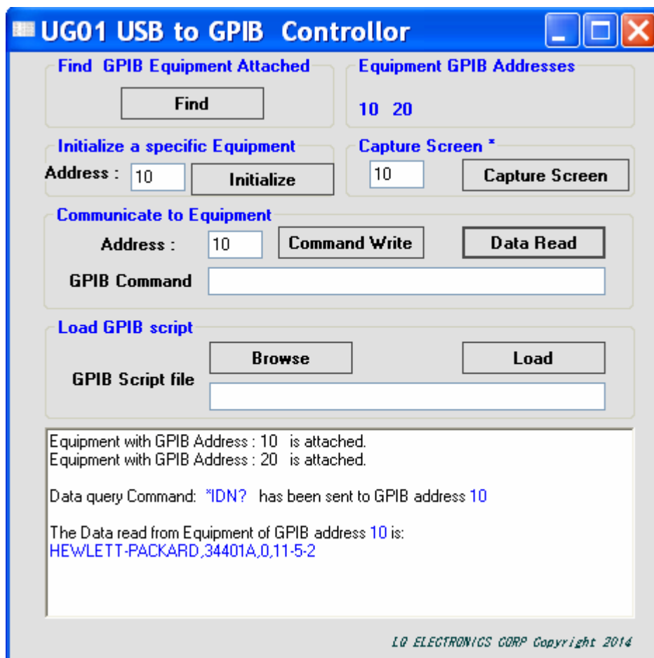
Fig. 1 UG01 Control Panel
