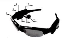
2: CH+/VOL+ 3: ON/OFF 4: CH-/VOI -5: Working indicator 6: Microphone 7: Headphone
