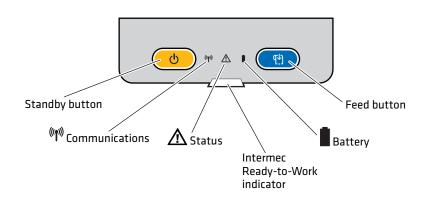
**PW50 Control Panel:** Use this illustration to familiarize yourself with the buttons and LEDs on the PW50.
