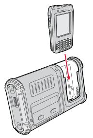
This illustration shows inserting a CN3. However, the PW50 is also designed for use with the CN3e, CK61, and CK61ex mobile computers.
