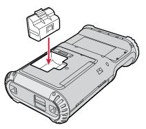
**3** Insert the edge of the battery under the lip of the PW50 and then push down until you hear the battery latch click.
