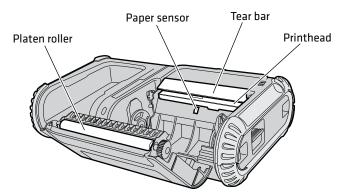
**PW50 Workboard Printer:** Identifying the parts of the PW50 to clean regularly.
