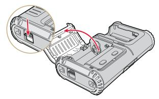
**2** Insert a roll of media. Make sure you load the media counterclockwise so that it pulls off the core from the bottom of the printer.
