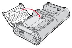
**5** Press down on the cover until it latches. The printer emits the hardware sound to tell you that the media door closed correctly.
