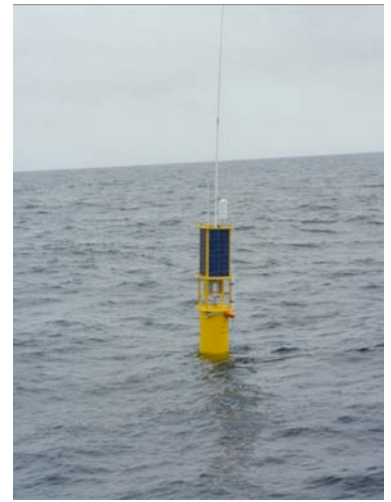
Shown here is SeaSonde bistatic transmitter mounted onto buoy off New Jersey coast.
