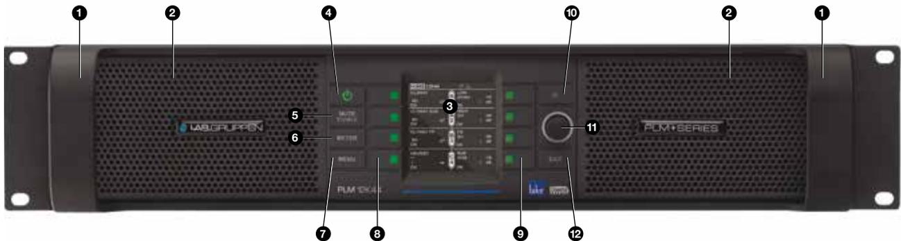
The front panel controls are clustered around a daylight readable LCD **3**, allowing adjustment and monitoring of the majority parameters and meters. The two clusters of controls on either side of the LCD include five dedicated function buttons **4 5 6 7 12**, eight dynamic function buttons with embedded LEDs **8 9** and a rotary data encoder **11**.
