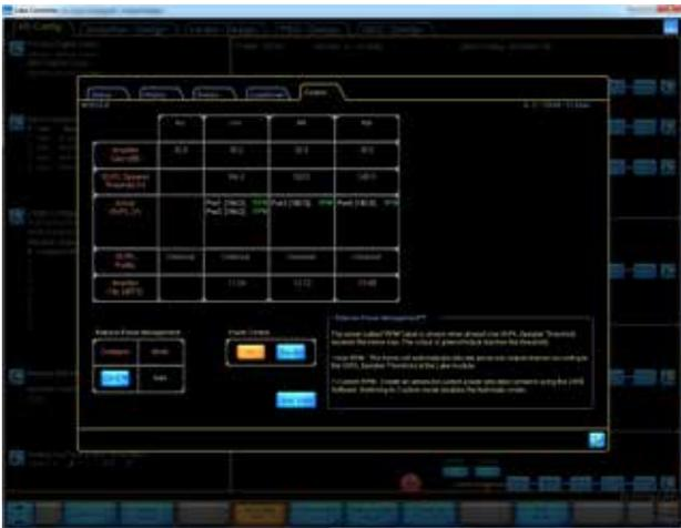
**Custom RPM:** The CAFÉ software allows users to create an advanced custom power allocation scheme. Switching to Custom mode disables the Automatic mode. When RPM is active an RPM icon will be displayed next to the “Actual ISVPL” values in the Events & Control section. Please find more information about this in documentation supplied with the CAFÉ software download.
