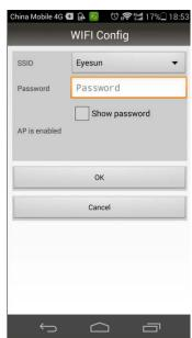
IV-Point-to-point AP direct connection(when you are in your home, and do not need the internet to control the bulb camera, you can just connect your mobile with the wifi sended out by the bulb camera to control the bulb camera in your home.)
