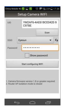
Step4 (Input the UID number or scan the QR code of this bulb camera Eyesun Step5 (Click SSID to choose the available WIFI signal
