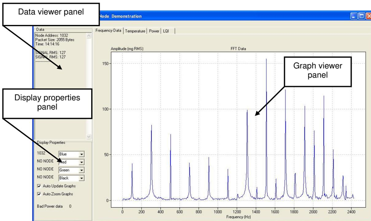
**Figure 2 – Perpetuum wSNAK Display Software showing the accelerometer FFT**
