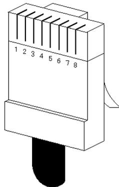
The pin numbers of the modular-jack for the connection diagrams below are based on the order described in the figure at the left.
