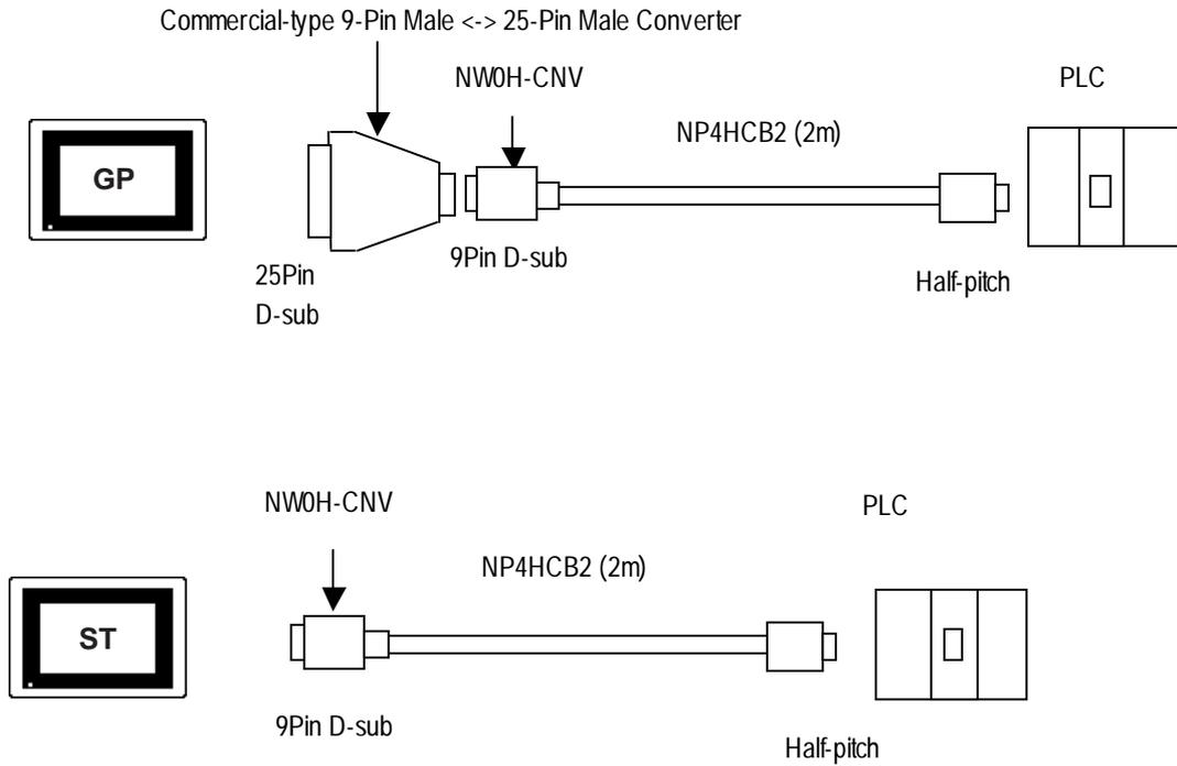
**■ D-sub 25Pin <-> D-sub 9Pin Conversion Adapter Specifications**
