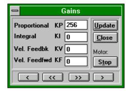
Select the Tuning Gains option from the main Options selection on the main menu. This will display the Gains dialog box. Type in the new value required for each gain term. The Update button will update all four gain values in the PTS. The Cancel button will remove the dialog
